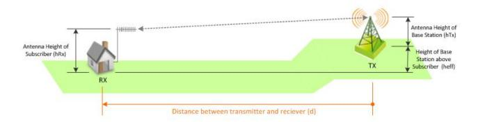
Figure 1. Model of major parameters impacting propagation (static environment).
