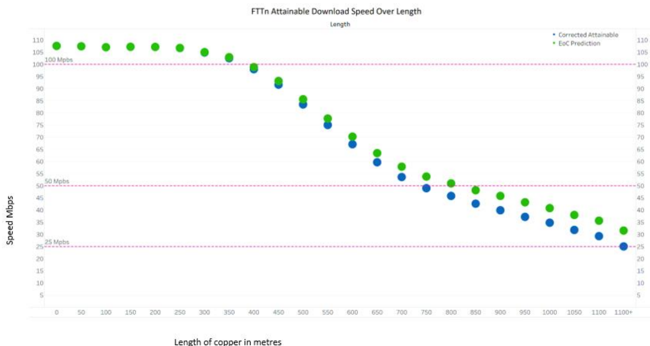
Diagram 9 – Copper Loop Length vs Download Speed
