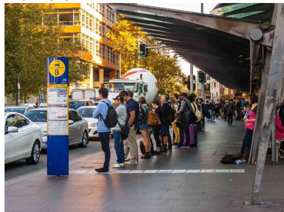
Railway Square Interchange boarding point blade lacks tactile markers
