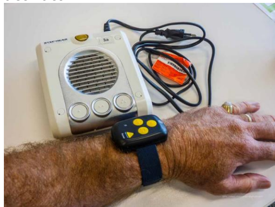
Step-Hear beacon and wrist activator
