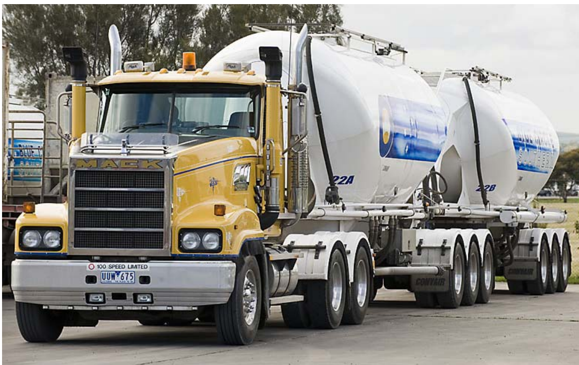
Figure 13: Mack B-double cement truck used in the trial
