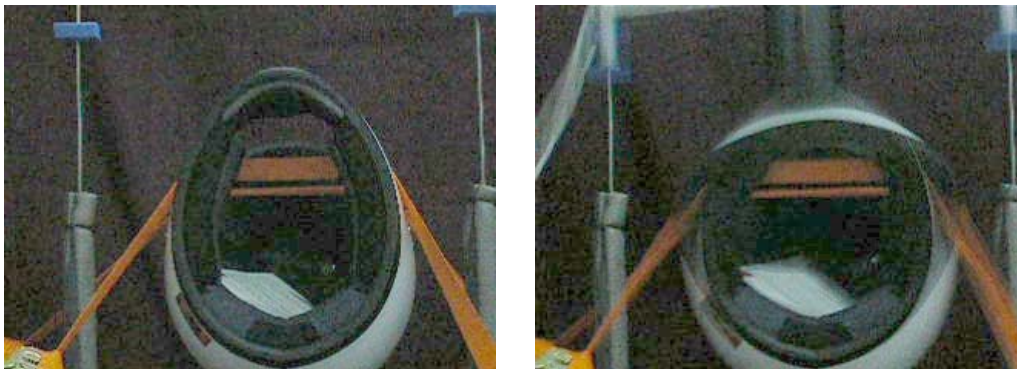
Figure 10 Snell chin bar test on first sample: helmet before impact (left) and at maximum chin bar deflection (right) of approximately 50 mm.
