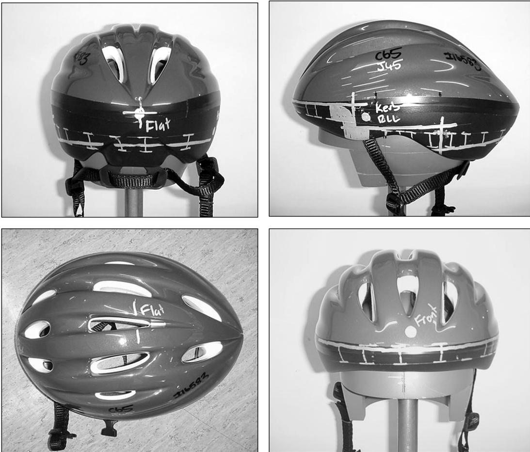
**Figure 5.3.** Diagram of a headform showing the position of the five impact test sites.
