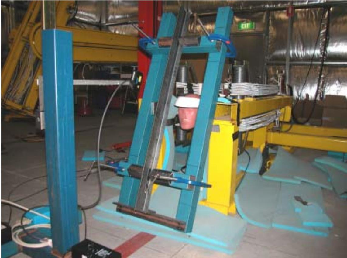
Figure 3-3 Test set-up with the headform, headband and beam in position prior to a test.
