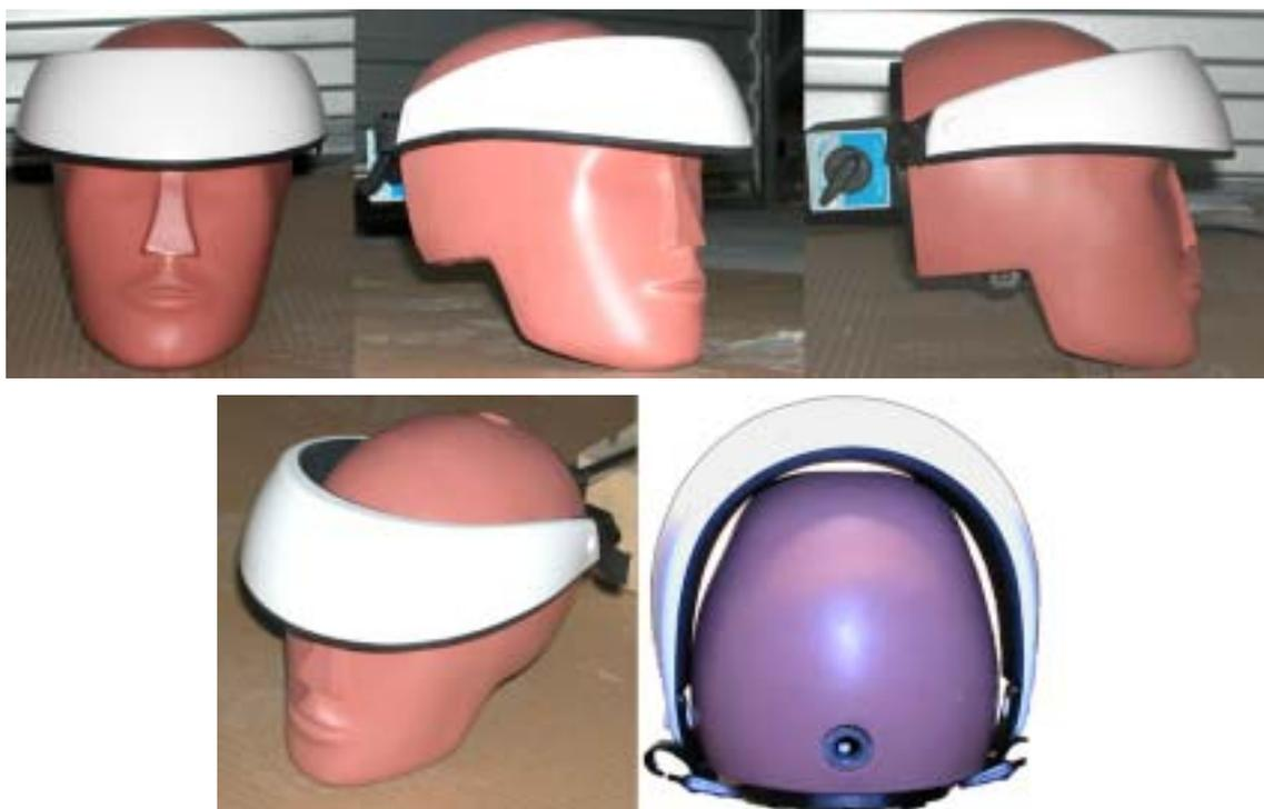
Figure 3-4 The headband attached to the headform. The last image shows the gaps between the headband and the headform that were filled with the insert.
