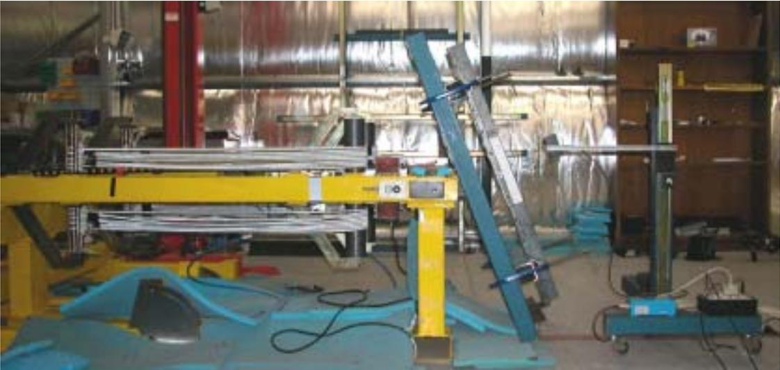
Figure 3-1 A photograph of the launcher and the beam fixed in position.
