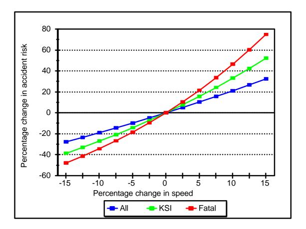
Figure 3.1. The percentage change in all accidents, killed and serious injury (KSI) accidents and fatal accidents (y-axis) as a function of percentage changes in mean speeds (x-axis). The steepness of the curve increases with accident severity. Based on Andersson and Nilsson (1997)
