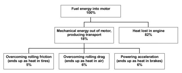
Figure 2.1. Energy consumption by petrol engines (from US DOT, 1998)
