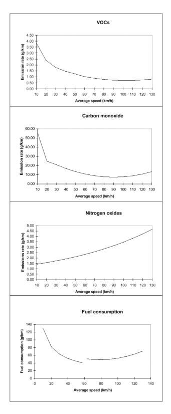
Figure 3.3. Typical emission rates for Volatile Organic Compounds (VOCs – elsewhere termed Hydrocarbons – HC), carbon monoxide, nitrogen oxides and fuel consumption as a function of average speed for passenger cars conforming to ECE 15-04 regulations (Eggleston et al., 1992, cited in Smith and Cloke, 1999).
