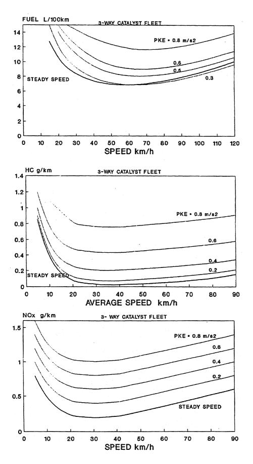
*Figure 3.4. Estimated effects of Positive Kinetic Energy (PKE) and average speed on fuel consumption, hydrocarbon (HC) emissions and NOx emissions. From Nairn et al., 1994.*
