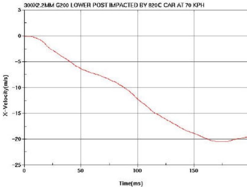
Figure 37 The velocity of occupant relative to the car for the post without cable
