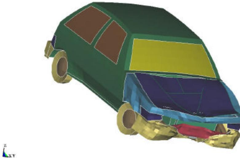
Figure 46 The deformed shape of the car
