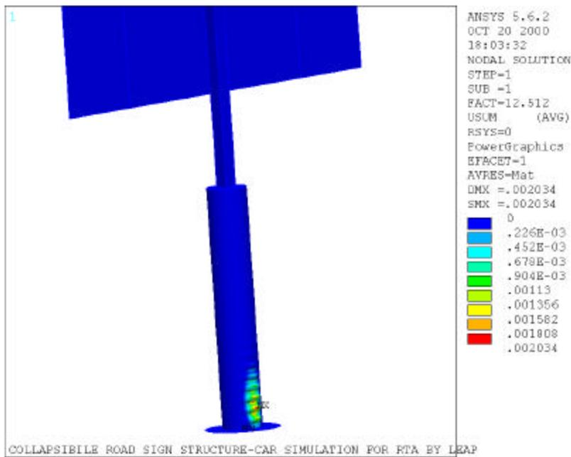
Figure 51 The buckling mode of the single cylinder post 300
