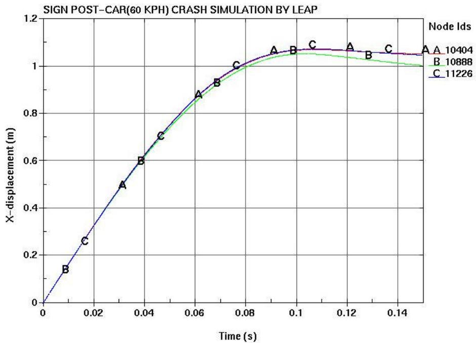
Figure 5 The displacement history at the nodes monitored
