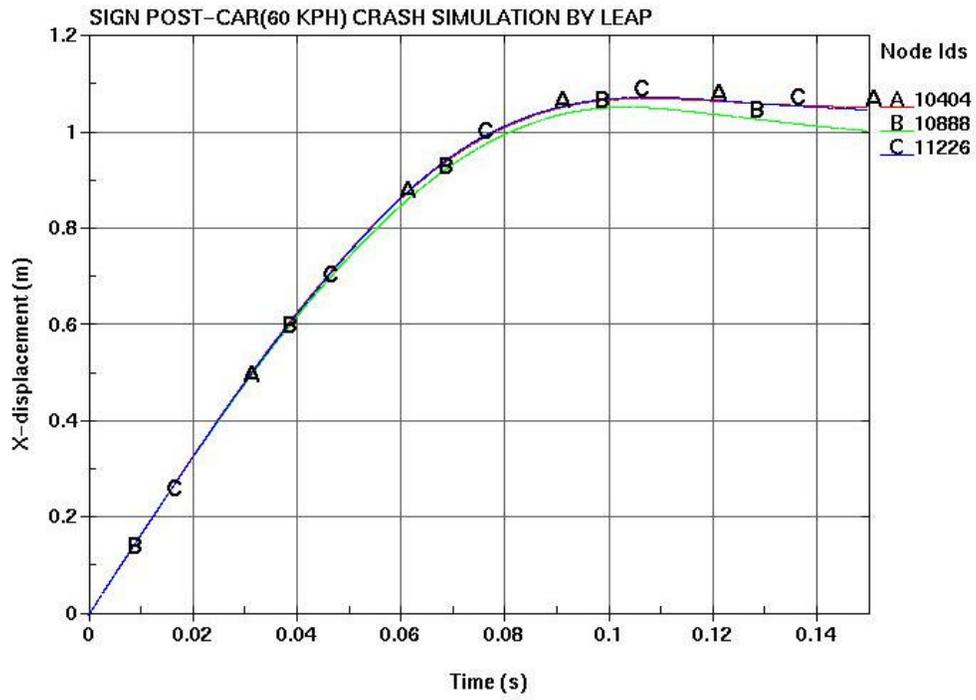
Figure 10 The displacement history at the nodes monitored
