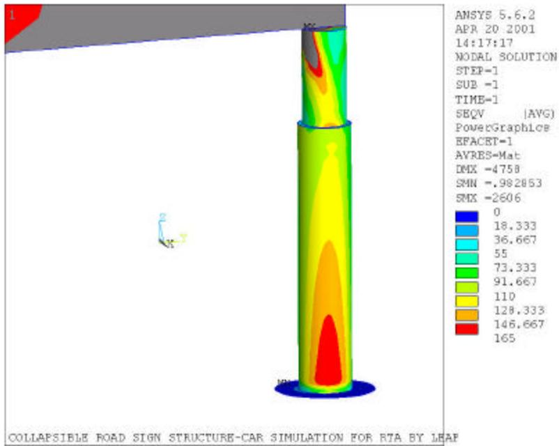
Figure 18 The Von-Mises stress on the shorter single post360
