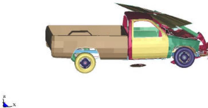
Figure 59 The truck movement after the crash for the post without cable
