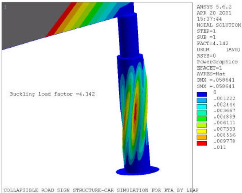
Figure 25 The buckling mode of the single cylinder post 400
