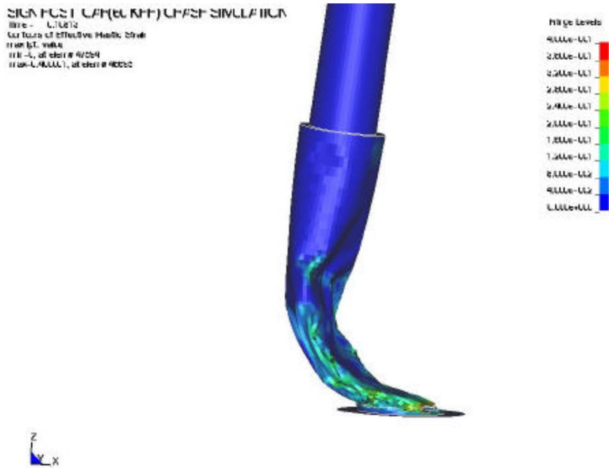
Figure 4 The plastic strain and the deformed shape of the post after impact
