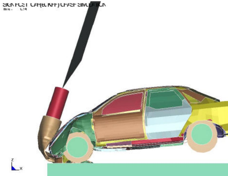
Figure 22 The deformed shape of the car and the post (shorter post400)
