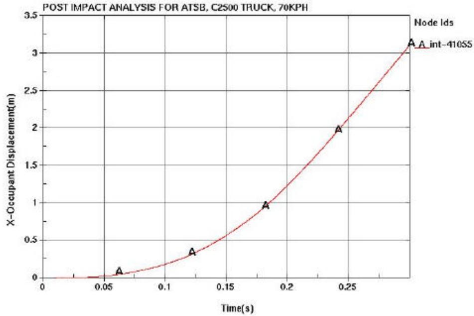
Figure 58 The displacement of the occupant relative to the car for the post with cable
