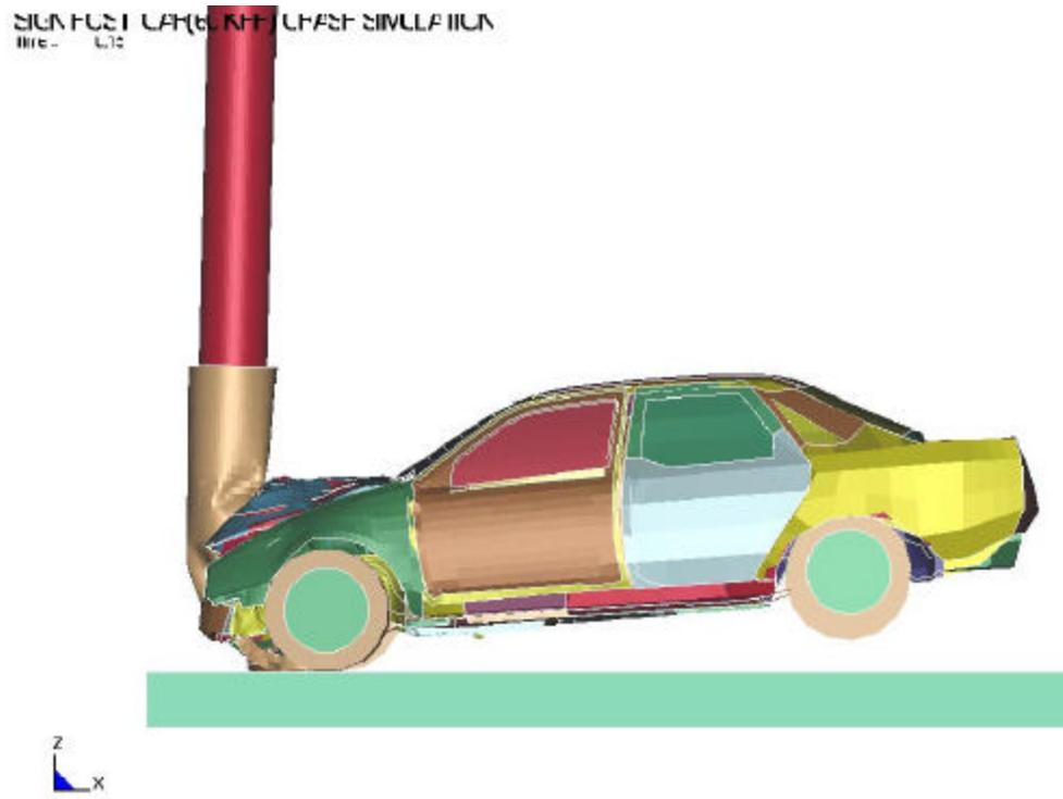
Figure 8 The deformed shape of the post 450-250-g350 and the car
