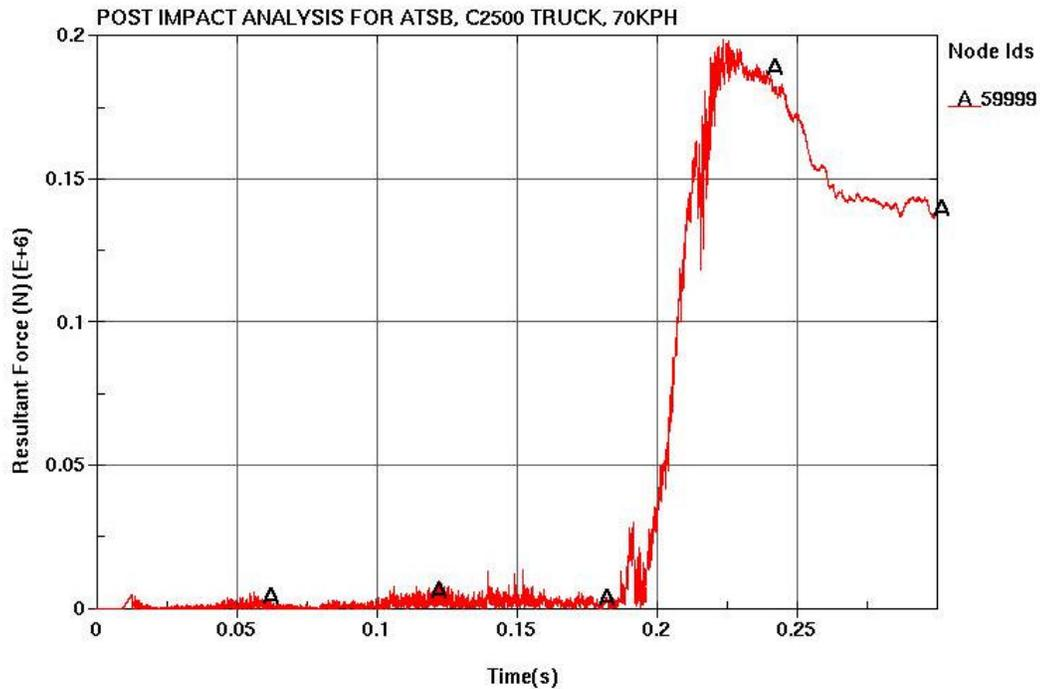
Figure 62 The force on the cable.
