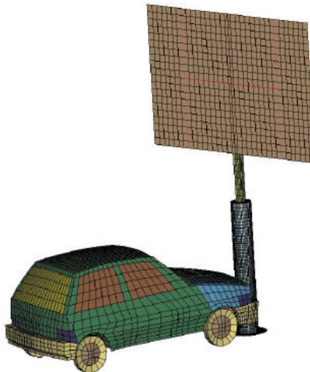
Figure 34 The finite element model of signpost (stage 4) and the colliding car
