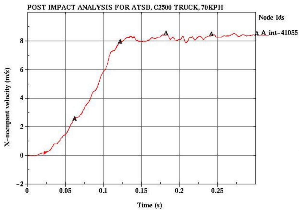
Figure 55 The velocity of the occupant relative to the truck for the post without cable
