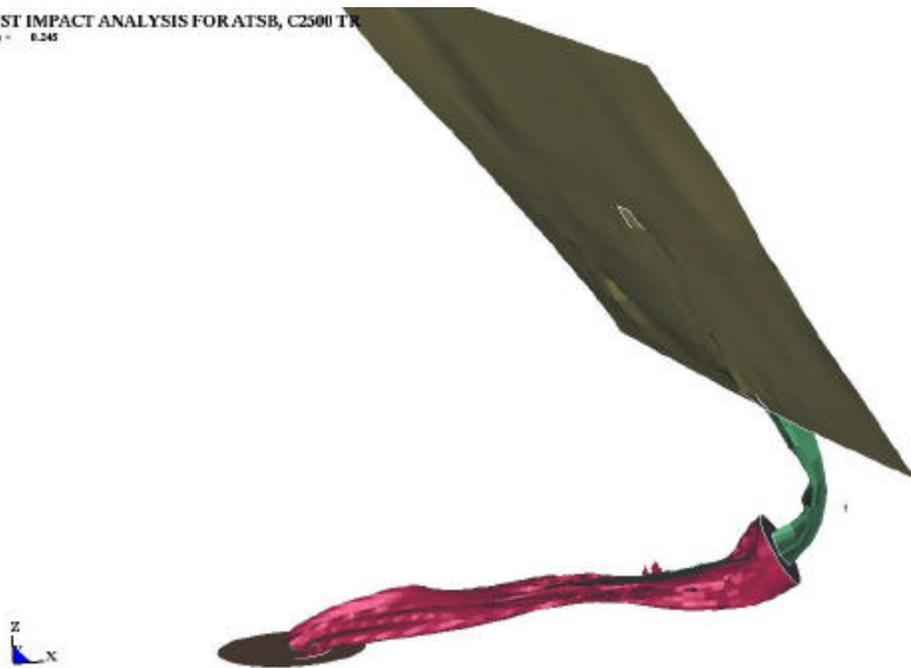
Figure 61 The deformed shape of the post with cable
