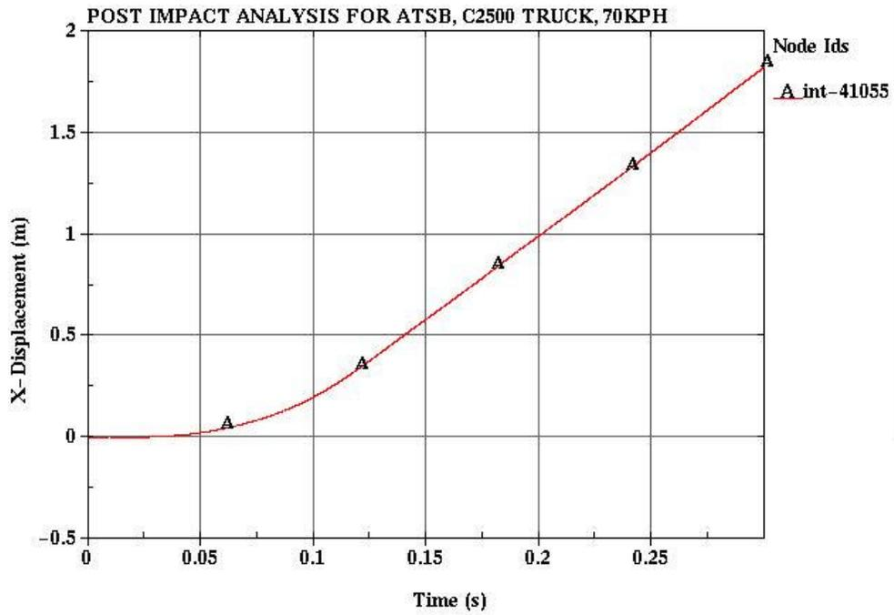
Figure 57 The displacement of the occupant relative to the car for the post without cable
