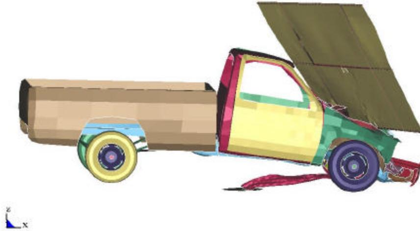
Figure 60 The deformed shape of the post and the truck for the post with cable
