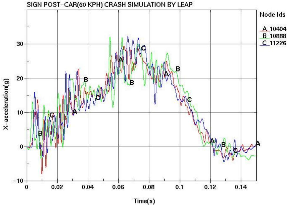
Figure 12 The acceleration history at the nodes monitored
