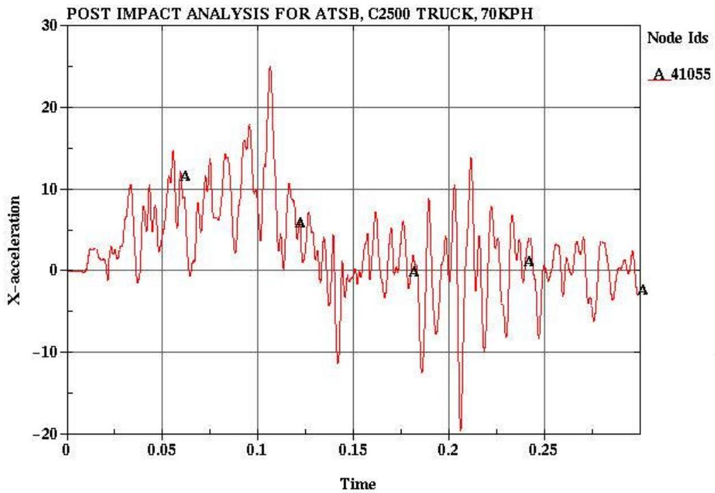
Figure 53 The acceleration history of the truck CG for the post without cable
