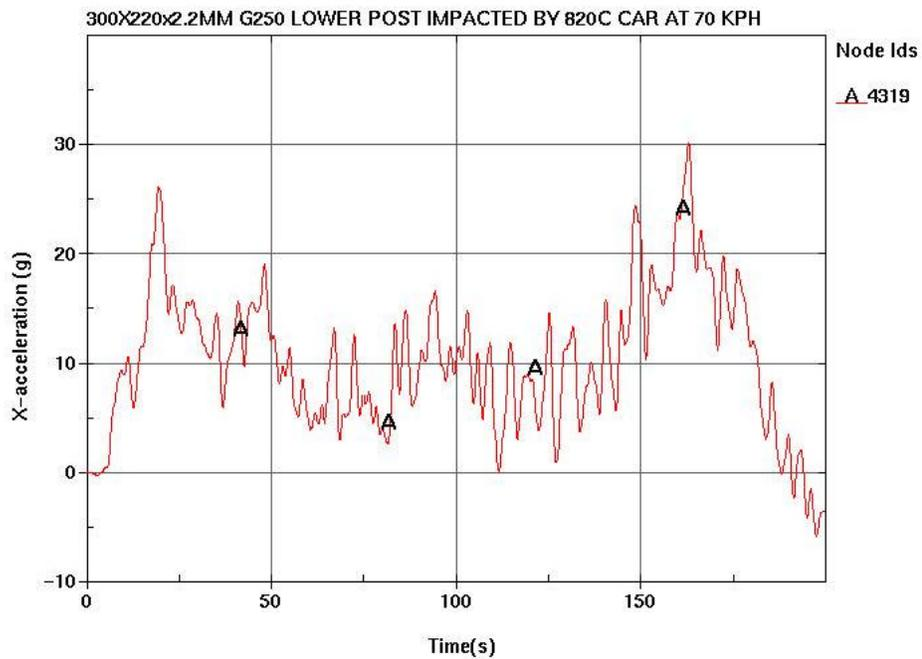
Figure 48 The acceleration history of the car CG for the taller cylinder post
