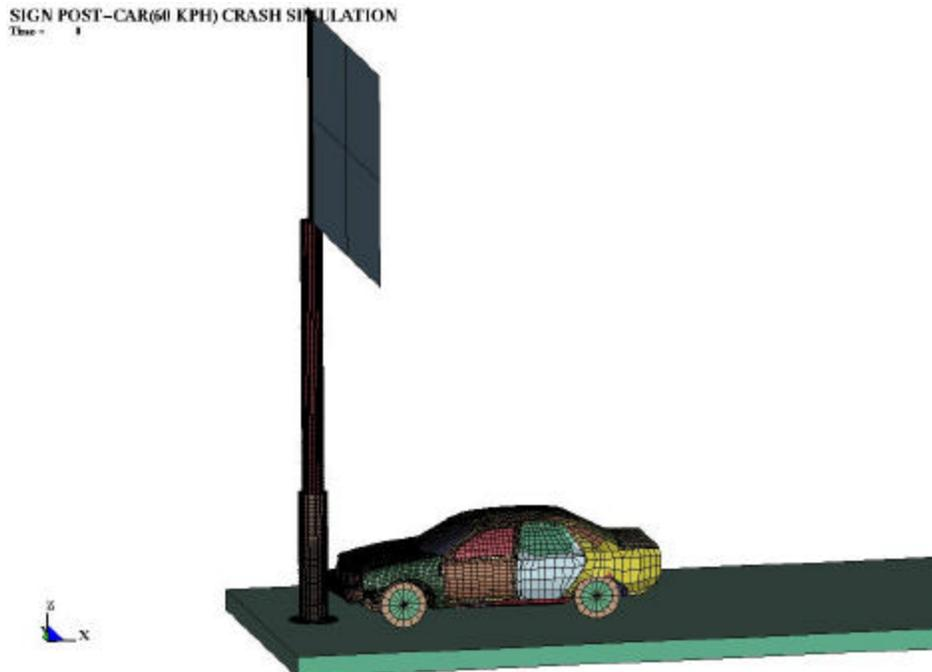
Figure 1 The finite element model of the signpost and the colliding car
