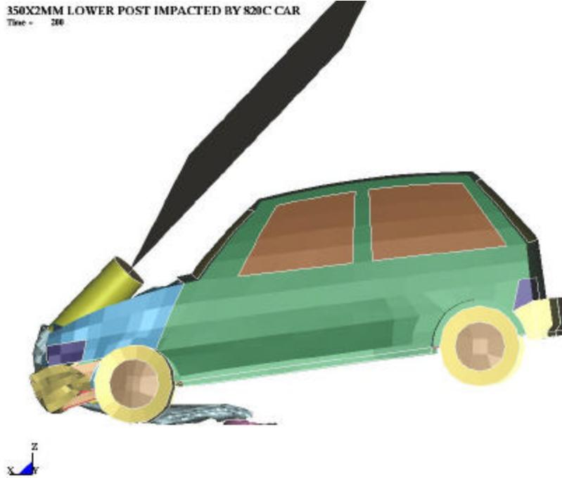
Figure 32 The deformed shape of the post grade 250 and the car
