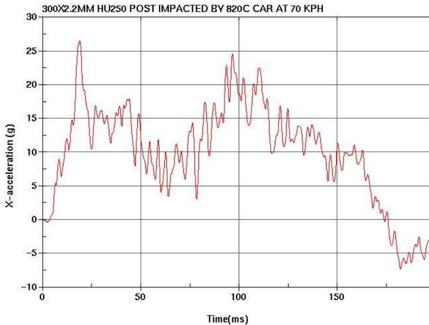
Figure 35 The acceleration history of the car CG for the post without cable
