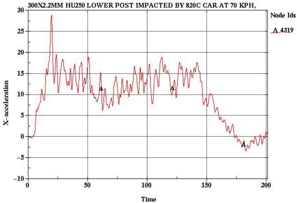
Figure 36 The acceleration history of the car CG for the post with cable
