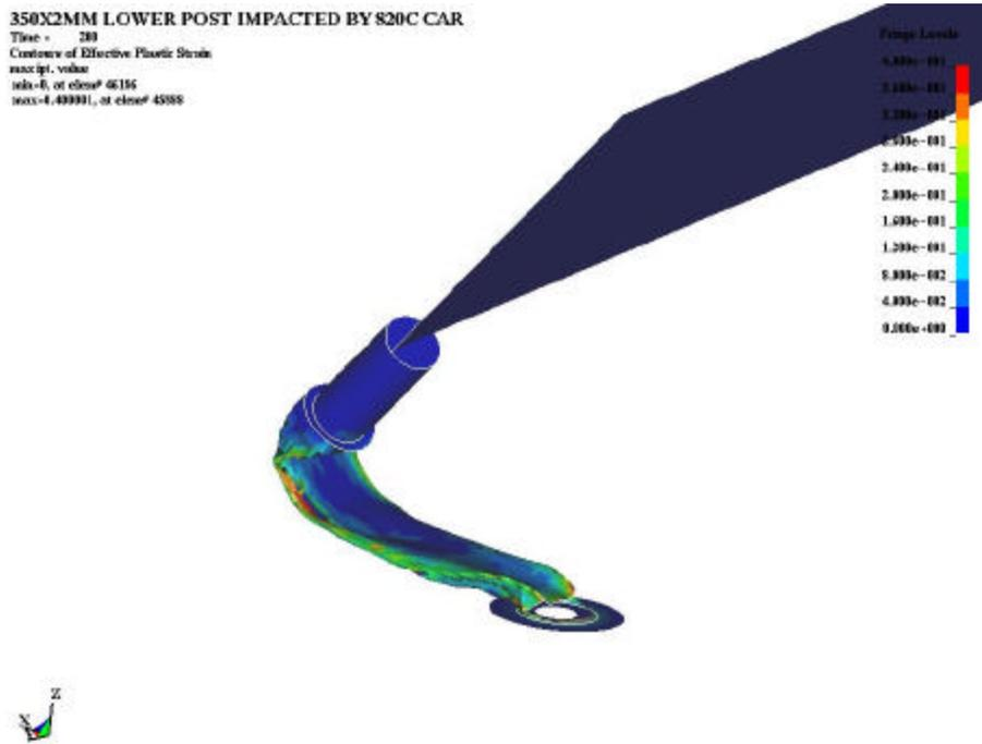
Figure 33 The deformed shape and the plastic strain of the post grade 250
