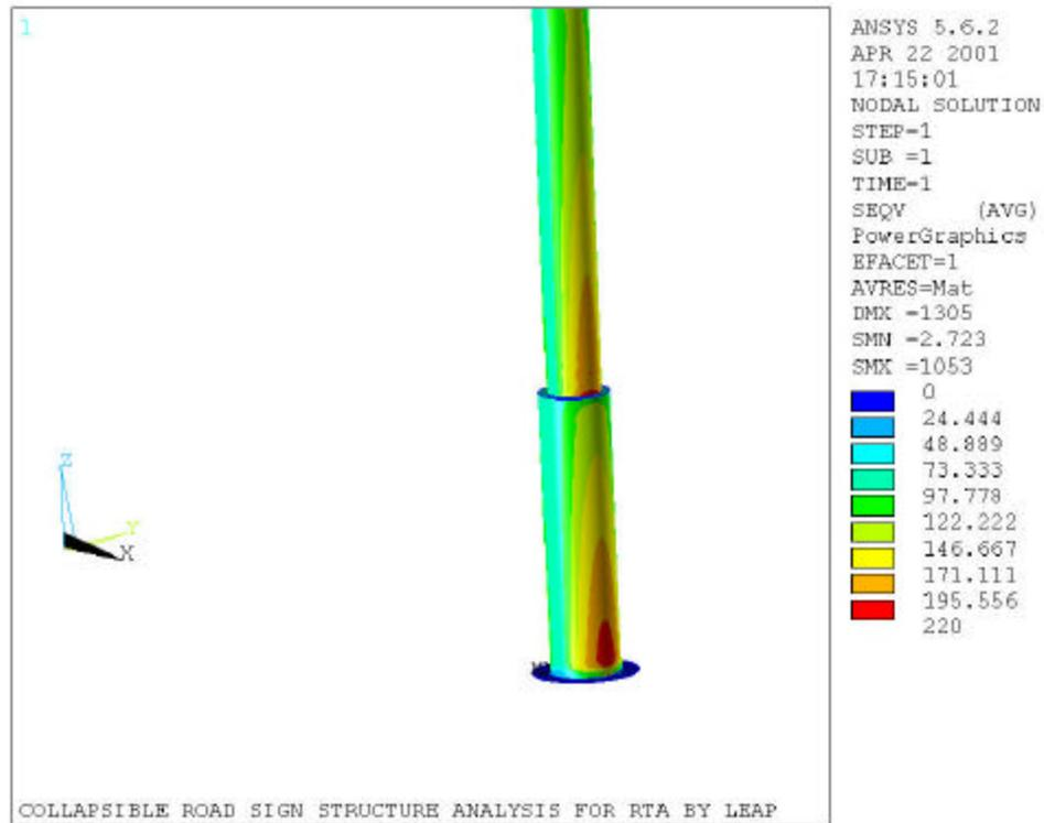
Figure 14 Von Mises stress on the 450-250 post
