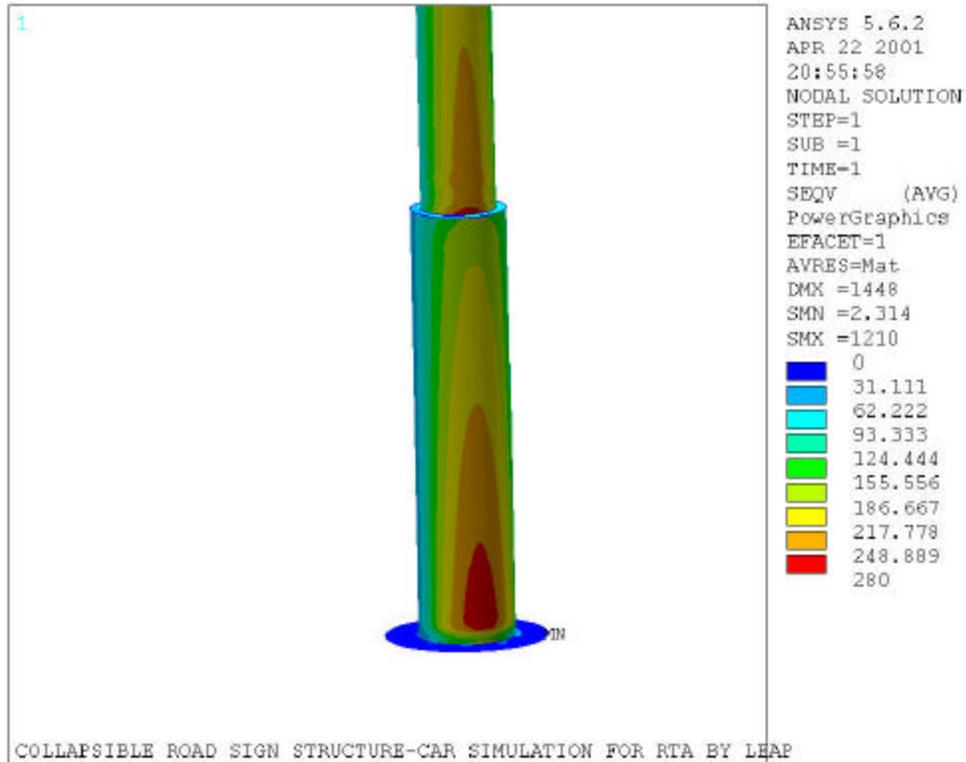
Figure 13 Von Mises stress on the 400-200 post
