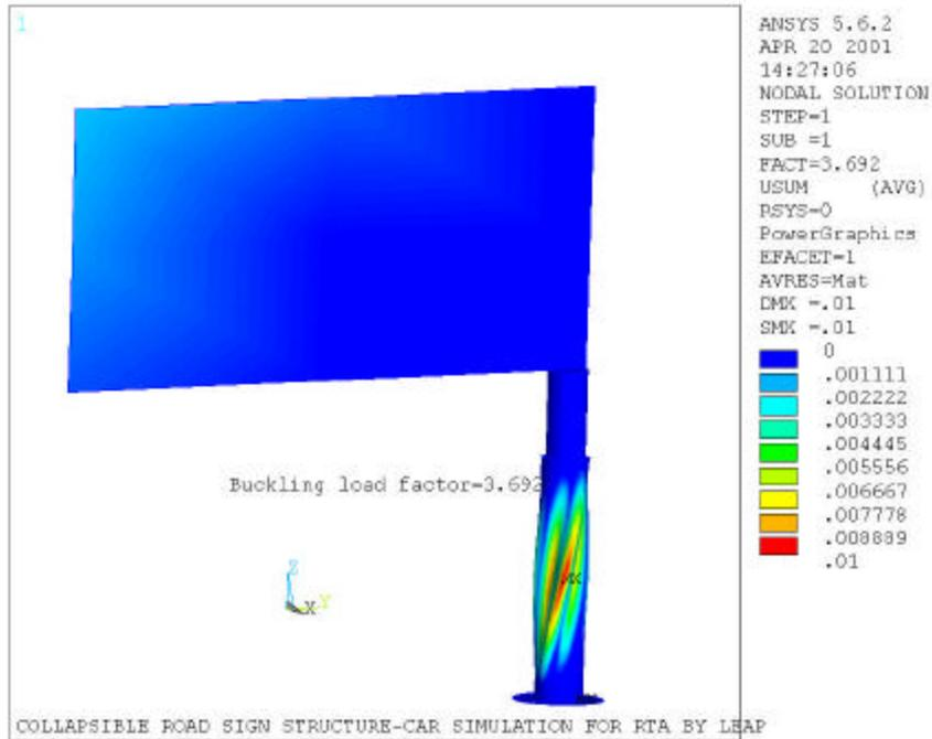
Figure 24 The buckling mode of the single cylinder post 360
