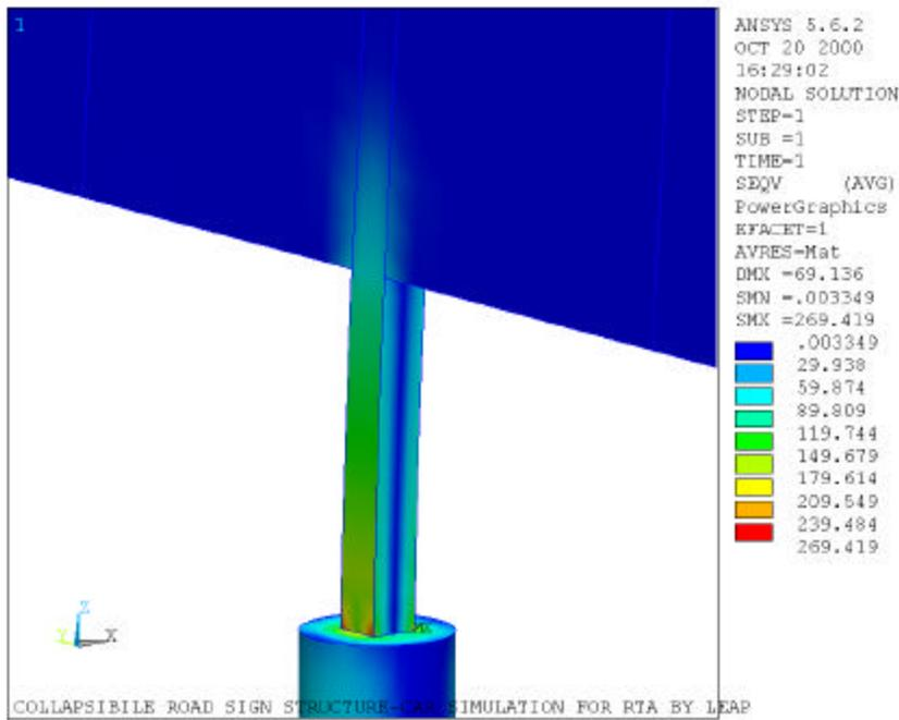
Figure 50 The Von-Mises stress on the extension post 100x100x5
