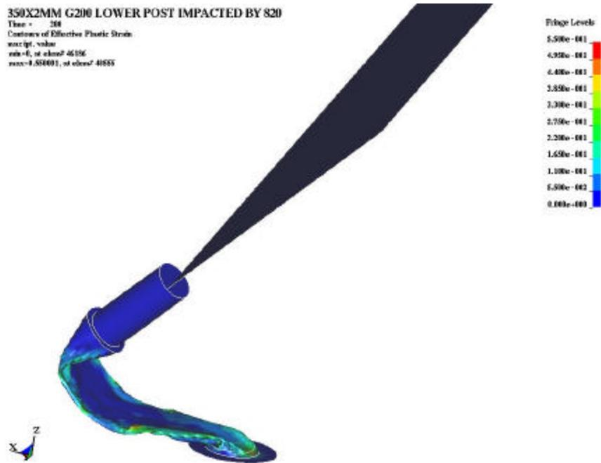
Figure 28 The plastic strain and the deformed shape of the post after impact
