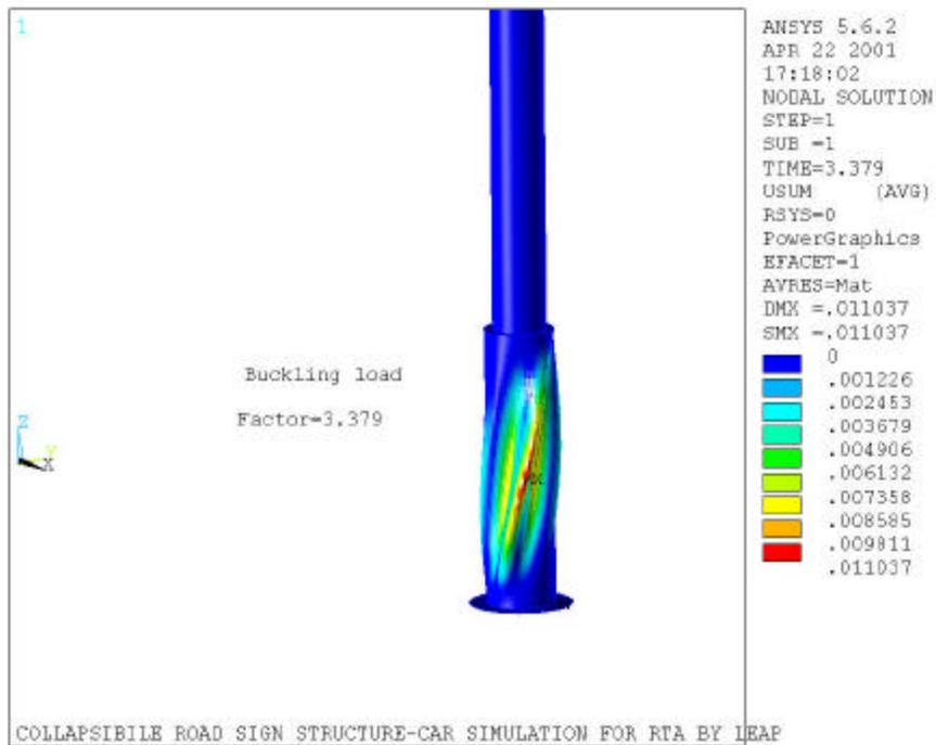
Figure 16 The first buckling mode of the signpost 450-250
