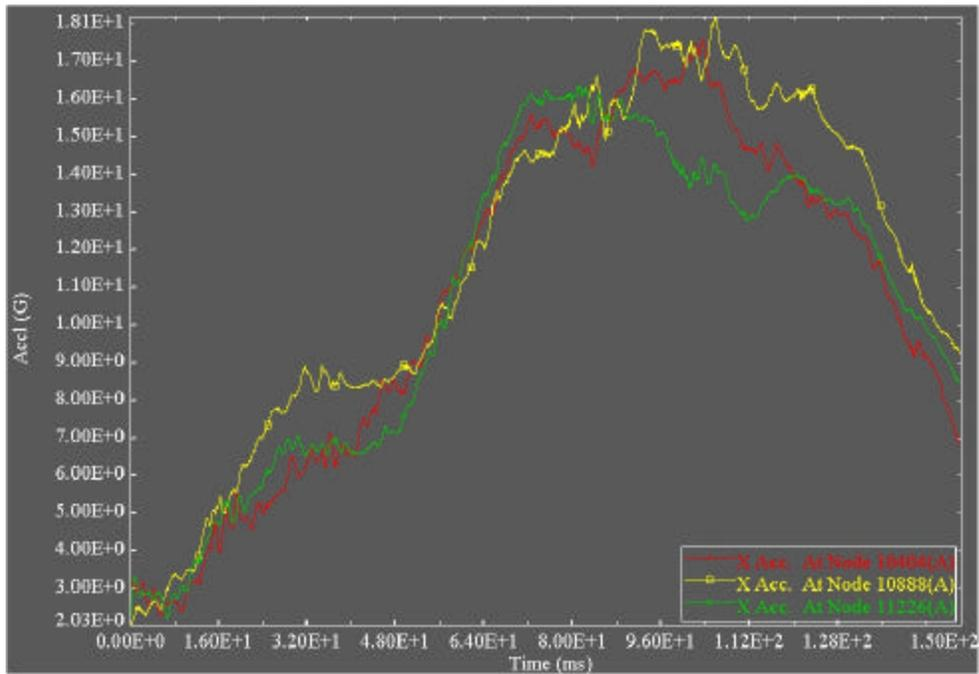
Figure 20 The acceleration of the car impact to a shorter single cylinder post360
