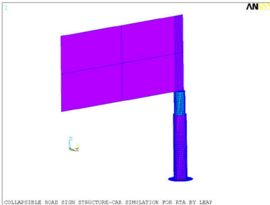
Figure 17 The FE model of the shorter post
