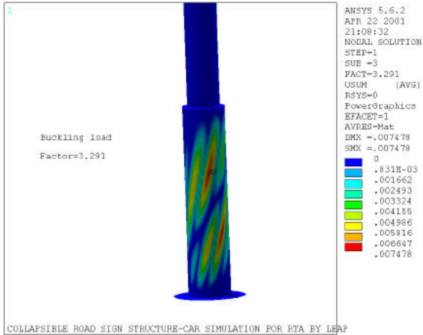
Figure 15 The first buckling mode of the signpost 400-200
