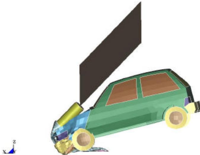
Figure 27 The deformed shape of the post and the car
