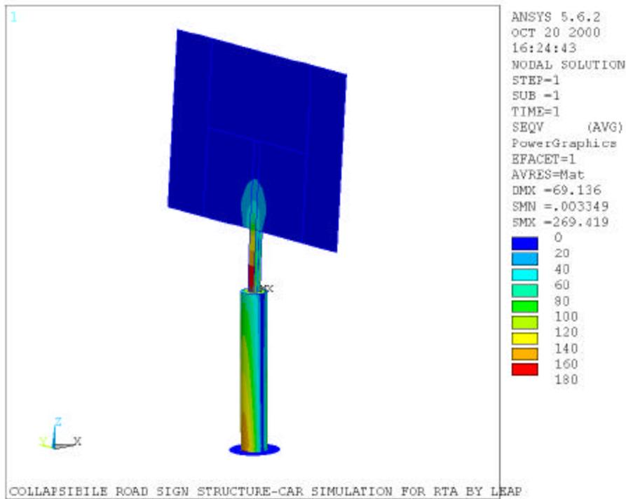
Figure 49 The Von-Mises stress on the single cylinder post300
