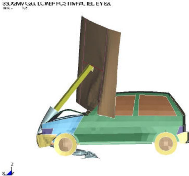
Figure 47 The deformed shape when only sign face centre was clamped.
