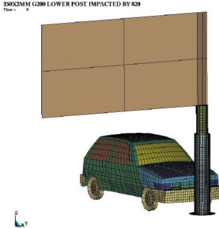
Figure 26 The finite element model of the signpost and the colliding car
