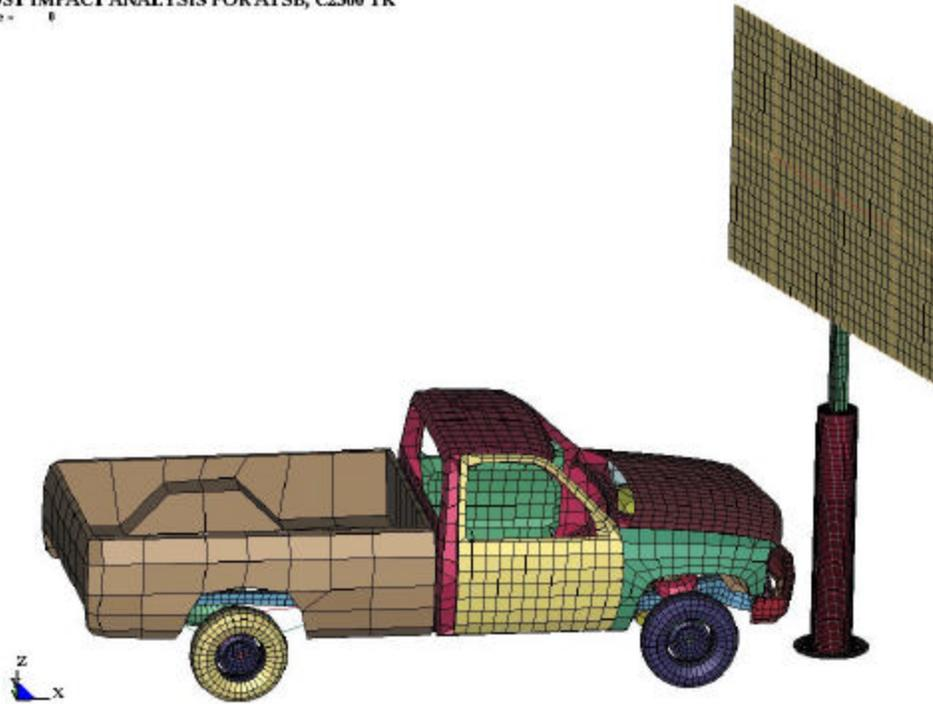
Figure 52 The finite element model of the signpost and the colliding car
