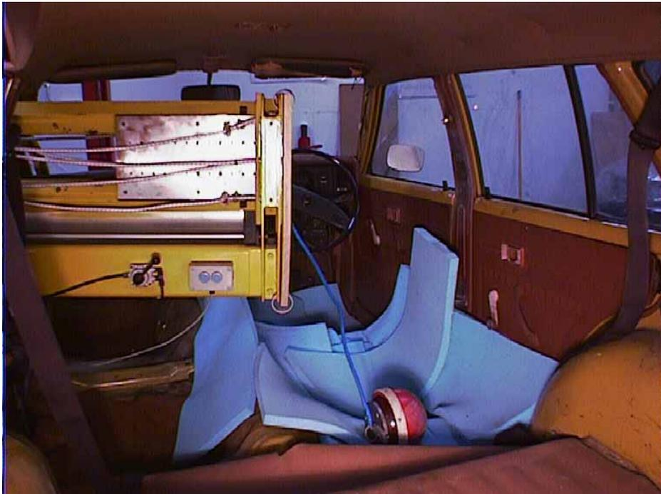
Figure 5-1 Test setup used in CR193. The photo was taken immediately after a test (Note that the RARU headform was used in the tests reported on in this report, not the EEVC WG10 headform as shown).
