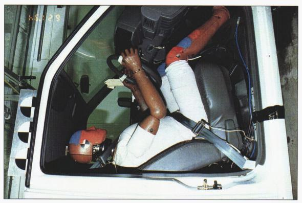
B4028 - Post-test driver's side closeup view
