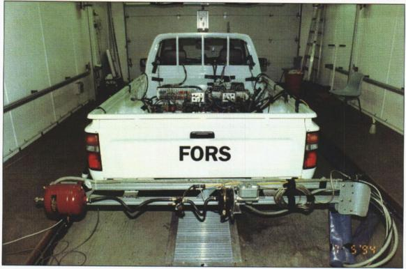
Typical test vehicle setup - rear view showing brake abort system and "umbilical cord" data cable (blue sheath).
