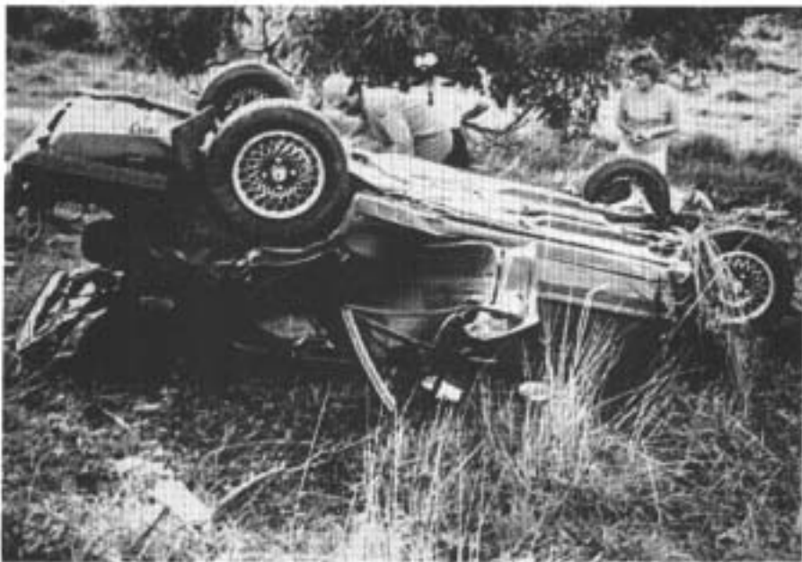
FIGURE A70: Crash 72. Final position of the car. Note extensive crushing of the roof into the occupant space.
