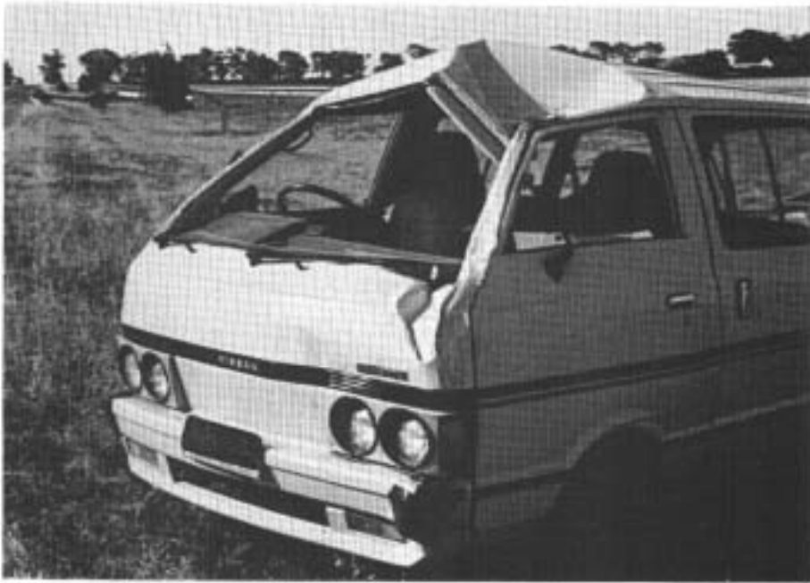
FIGURE A53: Crash 49. Final position of van showing damage sustained during rollover.
