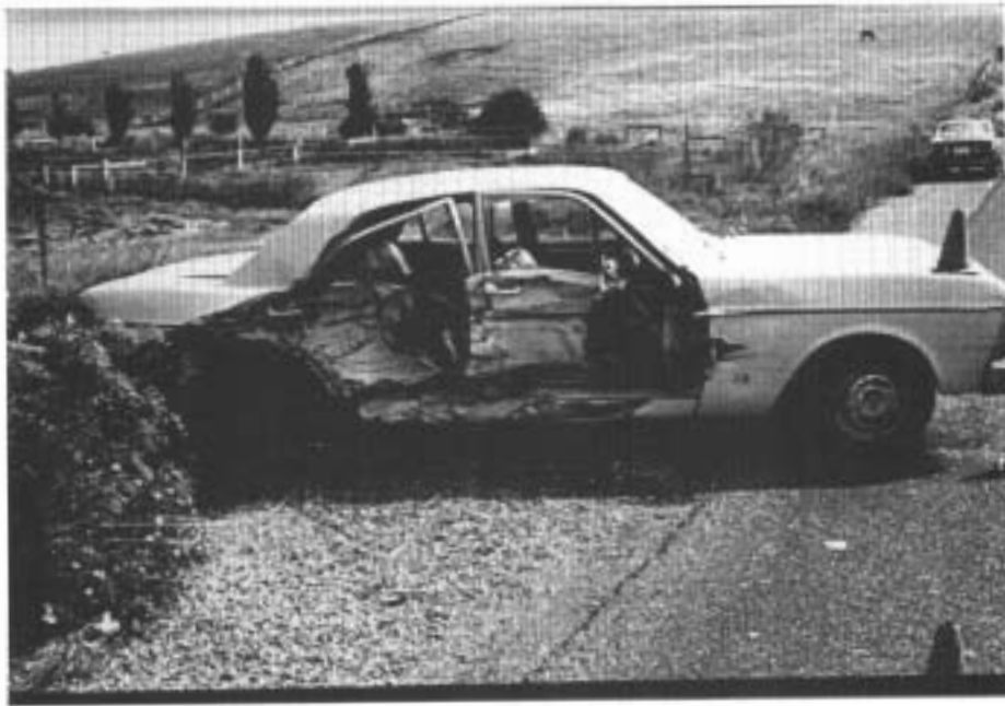
FIGURE A59: Crash 57. Final position of Ford Falcon and damage to right side.
