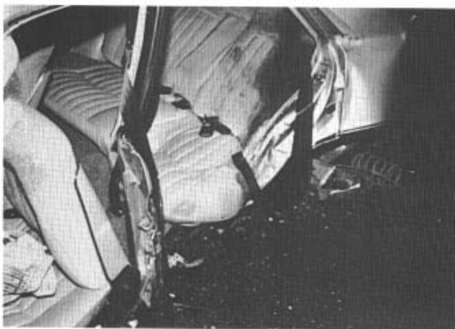
FIGURE A72: Crash 74. Left side of Sigma sedan which struck a tree on the left rear door. Note the intrusion into the rear seat occupant space. Left rear seat passenger was killed.
