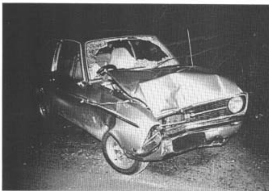
FIGURE A68: Crash 70. Final position of Ford Escort showing crash damage to front and right side. Note windscreen broken from contact by the unrestrained driver.
