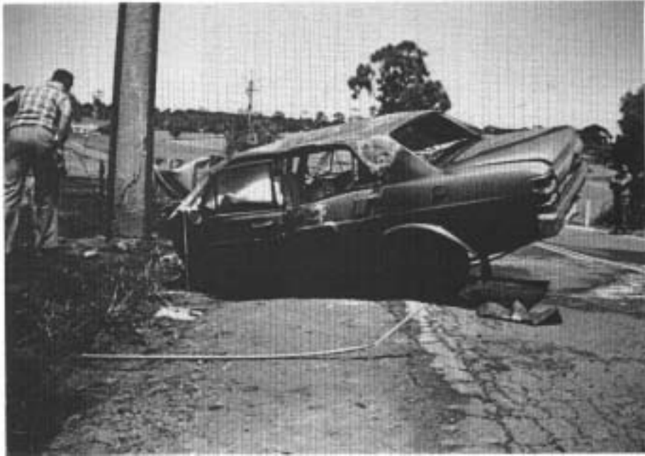
FIGURE A51: Crash 47. Final position of the car. Note damage to left front corner and scorching of the paint work from the fire which started after the impact.
