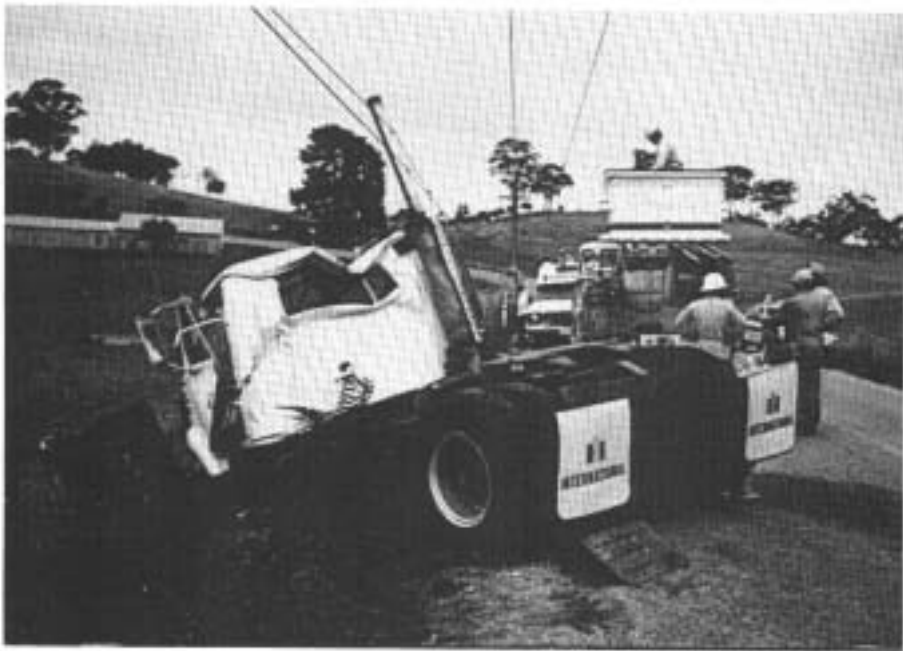
FIGURE A54: Crash 50. Final position of prime mover. Note deformation to right side of the roof due to impact with utility pole.
