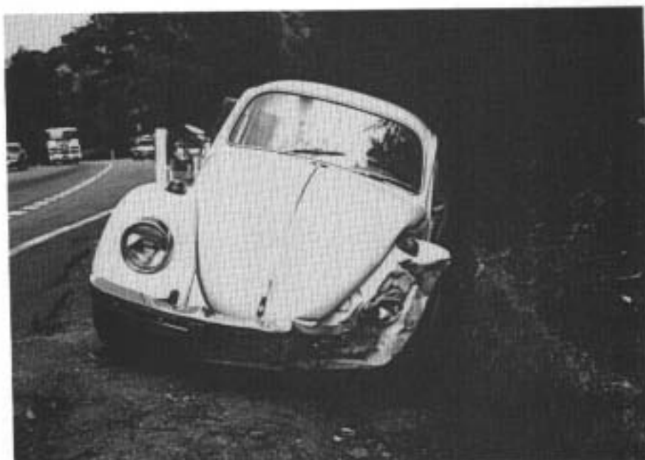
FIGURE A46: Crash 41. The final position of the car. Note damage to the left front corner due to impact with a concrete retaining wall.
