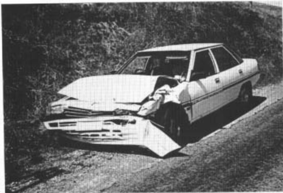
FIGURE A56: Crash 53. Frontal damage to Mitsubishi Magna.
