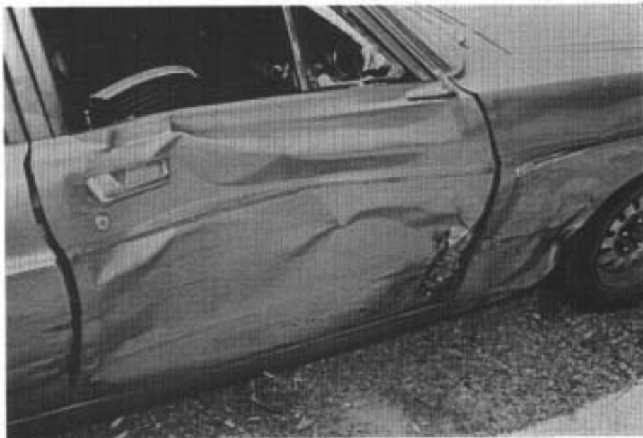
FIGURE A52: Crash 48. Damage to the right side of the car due to impact with the motorcycle and rider.
