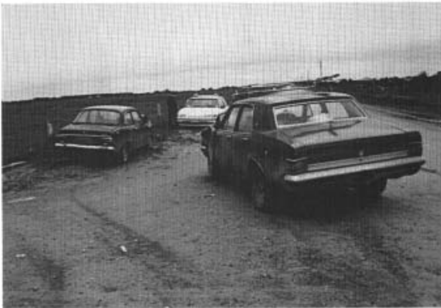
FIGURE A76: Crash 78. Final positions of Holden Premier sedan and Ford Escort sedan. Note skid marks indicating the vehicles' paths after impact.
