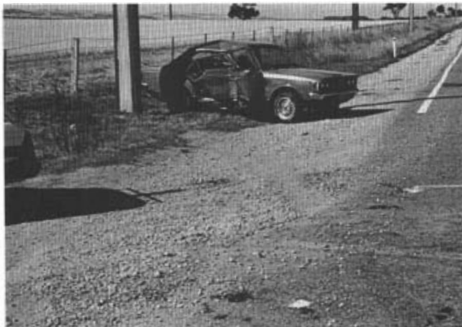
FIGURE A49: Crash 44. Final position of Toyota Corona. Note damage to right side and forward displacement of 'B' pillar due to impact with pole.
