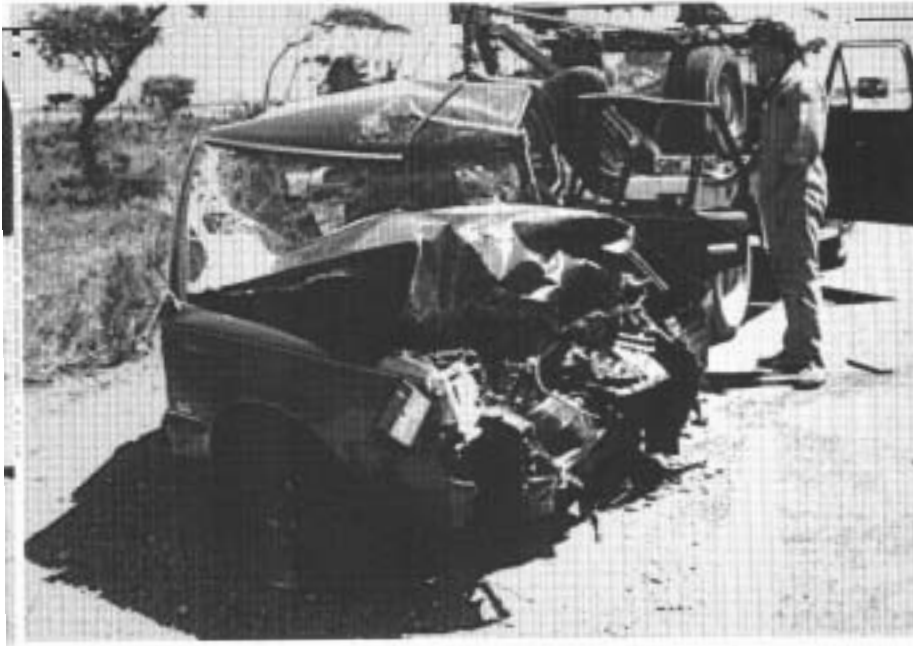
FIGURE A55: Crash 52. Frontal damage to Toyota Corona.
