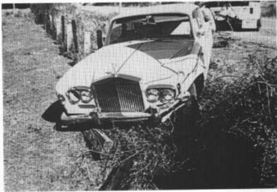
FIGURE A57: Crash 54. Final position of Rolls Royce, and frontal damage due to impact with fence post.
