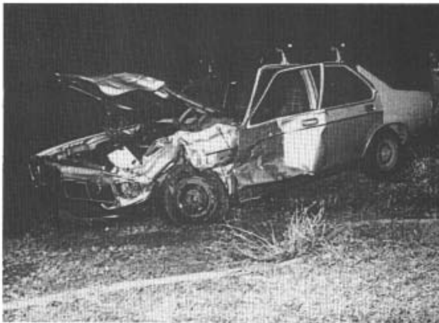
FIGURE A67: Crash 69. Final position of Holden Torana showing impact damage to left side.
