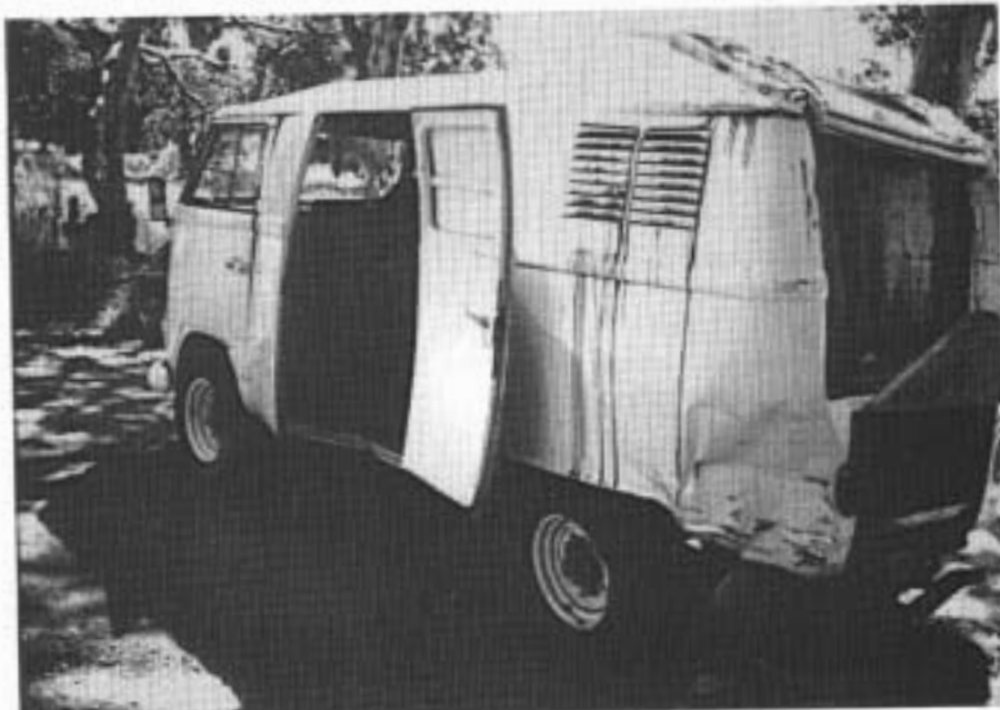
FIGURE A58: Crash 55. Damage to left side of van. Centre and rear doors opened during the rollover allowing the rear occupants to be ejected.
