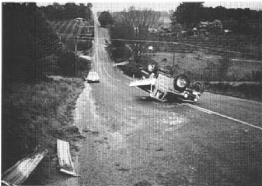
FIGURE A74: Crash 76. Final position of the utility. Note panels from the rear tray on the shoulder of the road.
