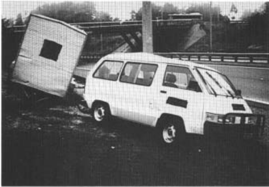
FIGURE A69: Crash 71. Final position of the van which came to rest against a non-frangible pole. Note the trailer which has become detached after breaking off the towbar from the van.
