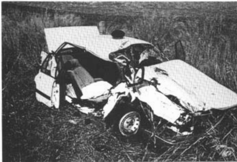
FIGURE A62: Crash 60. Final position of Holden Camira showing extensive damage to the right side due to impact with the semi-trailer.
