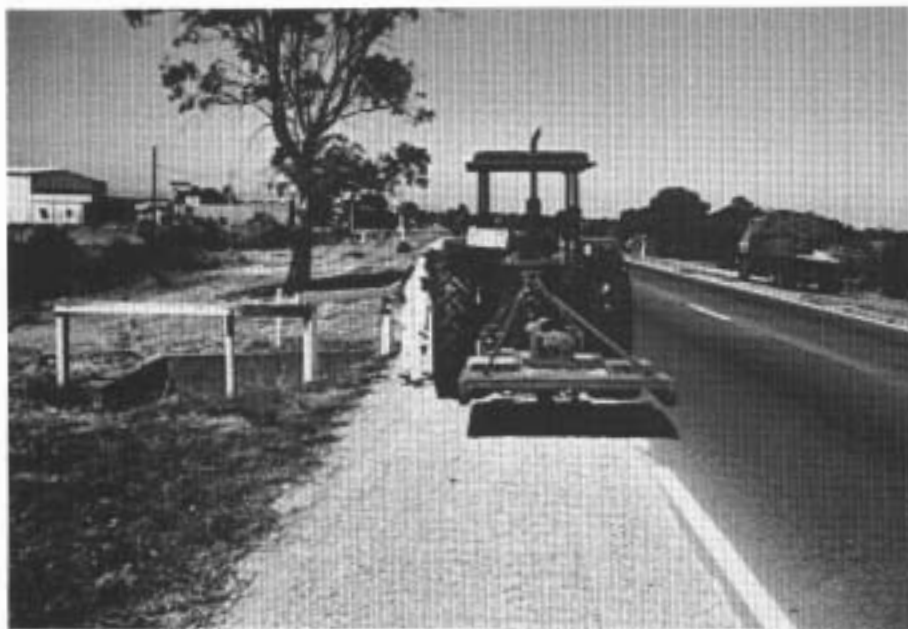
FIGURE A50: Crash 46. Tractor with mower attachment struck by motorcycle. The motorcycle contacted the right rear corner of the mower.
