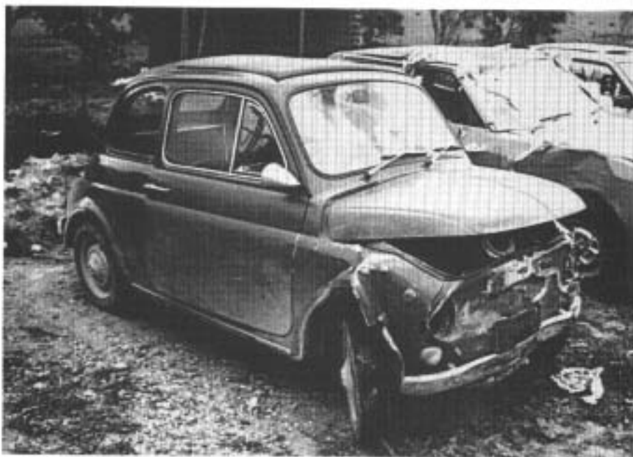
FIGURE A19: Crash 19. Impact damage to front of Fiat 500.
