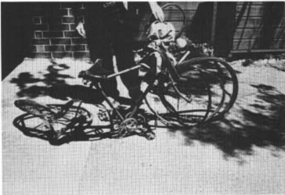
FIGURE A38: Crash 34. Damage to bicycle struck from the rear by a semi-trailer.
