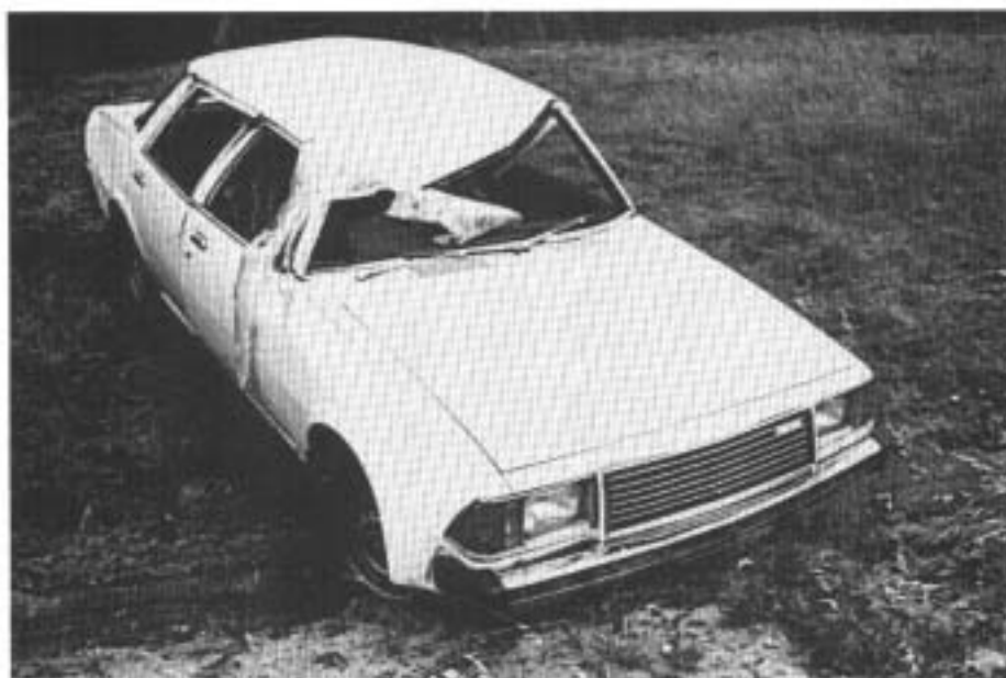
FIGURE A44: Crash 39. Final position of the car and damage to roof sustained during rollover.
