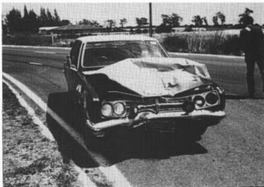
FIGURE A36: Crash 33. Final position of Holden Kingswood. Frontal damage due to striking right rear wheels of the trailer of a tray top truck.
