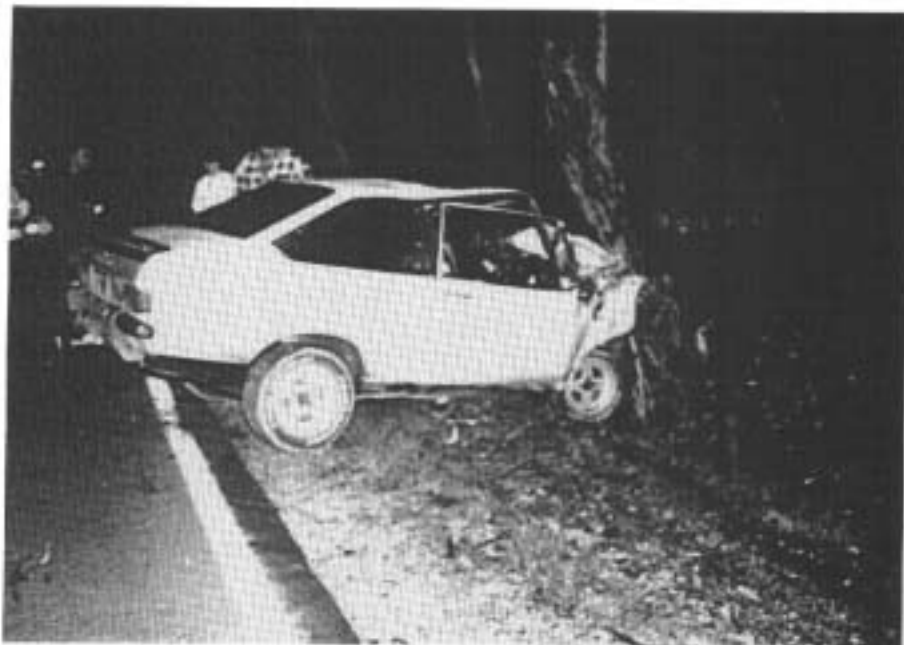
FIGURE A9: Crash 09. Final position of the car showing impact damage to the front right corner.
