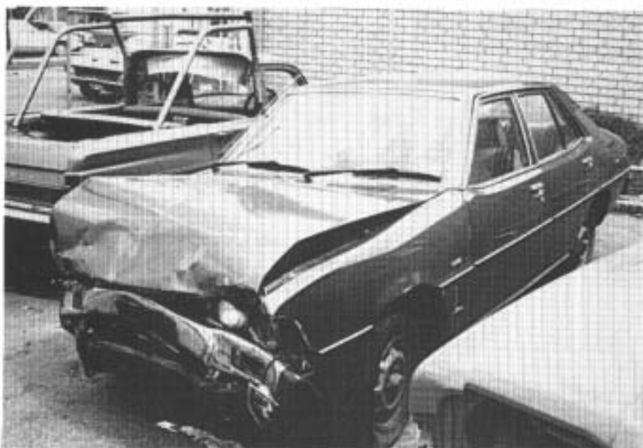
FIGURE AZO: Crash 19. Impact damage to front of Sigma sedan.
