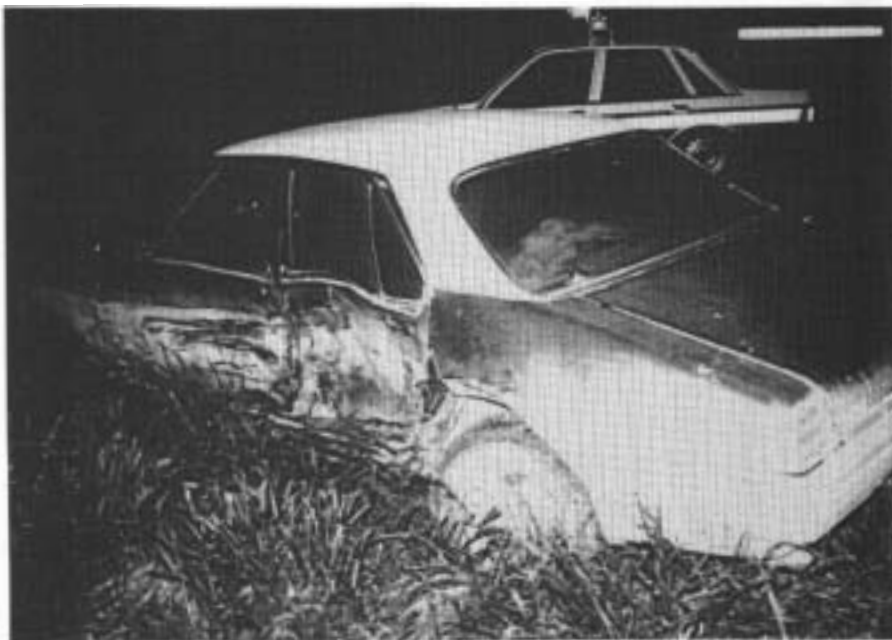
FIGURE A30: Crash 28. Holden Kingswood in its final position with damage to its left side.
