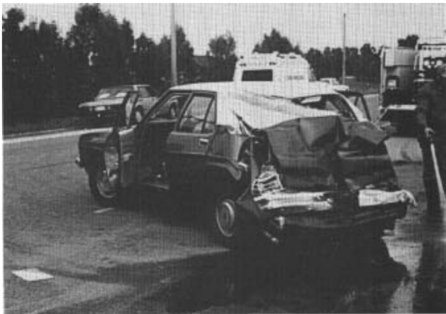
FIGURE A6: Crash 06. Impact damage to Holden Kingswood Sedan. Note impressions on the compressed boot from the bull bar of the semi-trailer.
