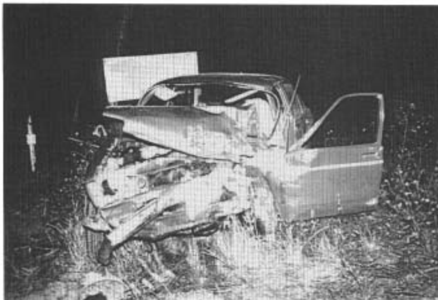
FIGURE A31: Crash 28. Holden Gemini in its final position with damage to the left front corner from striking Holden Kingswood.
