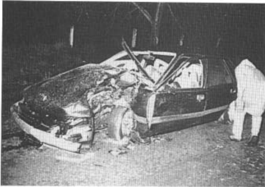
FIGURE A15: Crash 15. Final position of the car showing impact damage from striking a tree. Note distortion of door frame which was struck by the driver as he was ejected from the vehicle.
