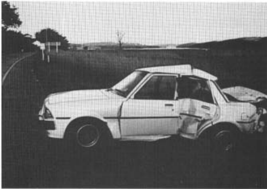
FIGURE A7: Crash 07. Final position of the car. Note impact damage to the left rear door and corner from impact with road sign.
