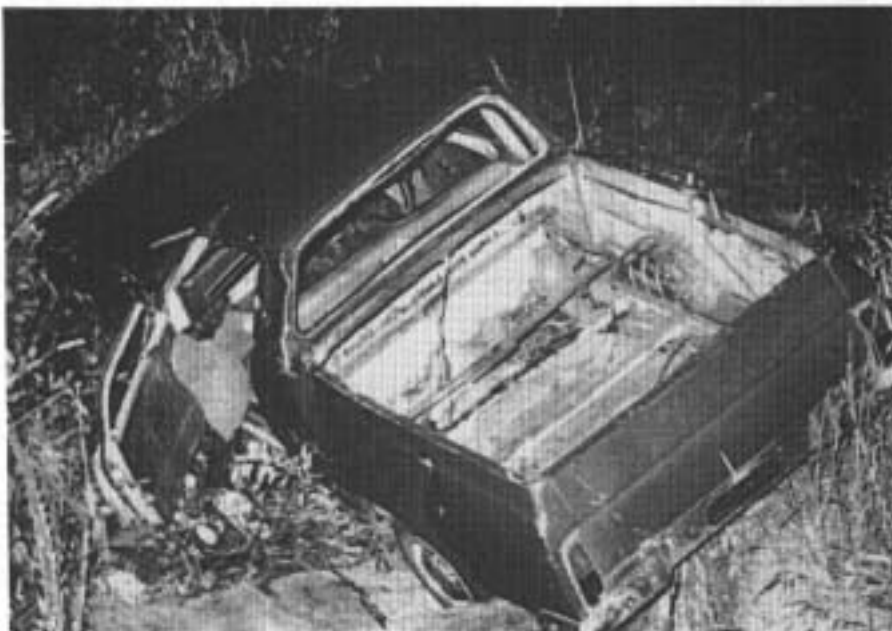
FIGURE A42: Crash 37. Final position of the utility. Note open left door through which two of the occupants, who both died, were partially ejected; and the severe rusting of floor pan of the rear load compartment.
