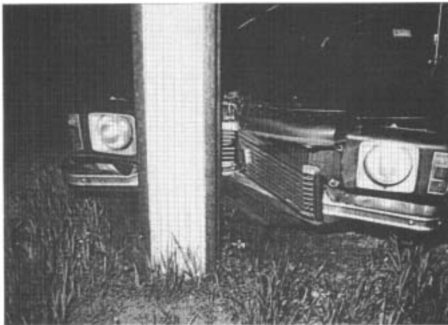
FIGURE A18: Crash 18. The final position of the car with impact damage to the front from impact with the pole.
