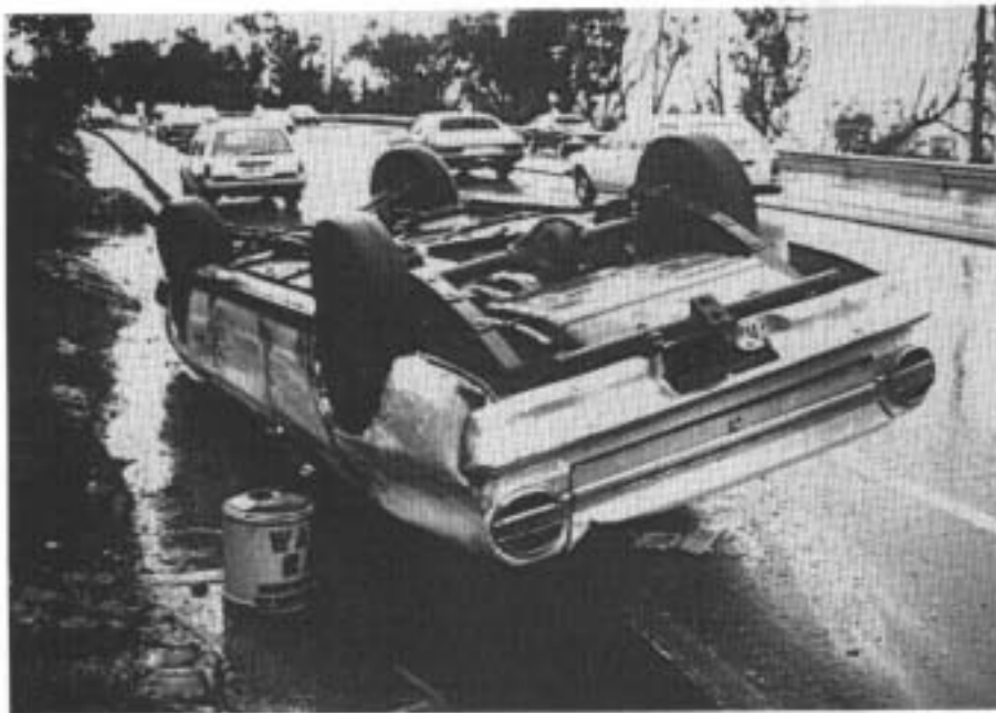
FIGURE A12: Crash 12. Final position of the car. Note scrape marks down right side from impact with embankment.
