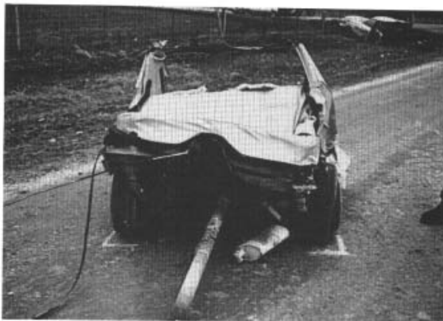
FIGURE A1: Crash 01. Detached rear section of Datsun 120Y Sedan with front section and Unit 1 visible in background.
