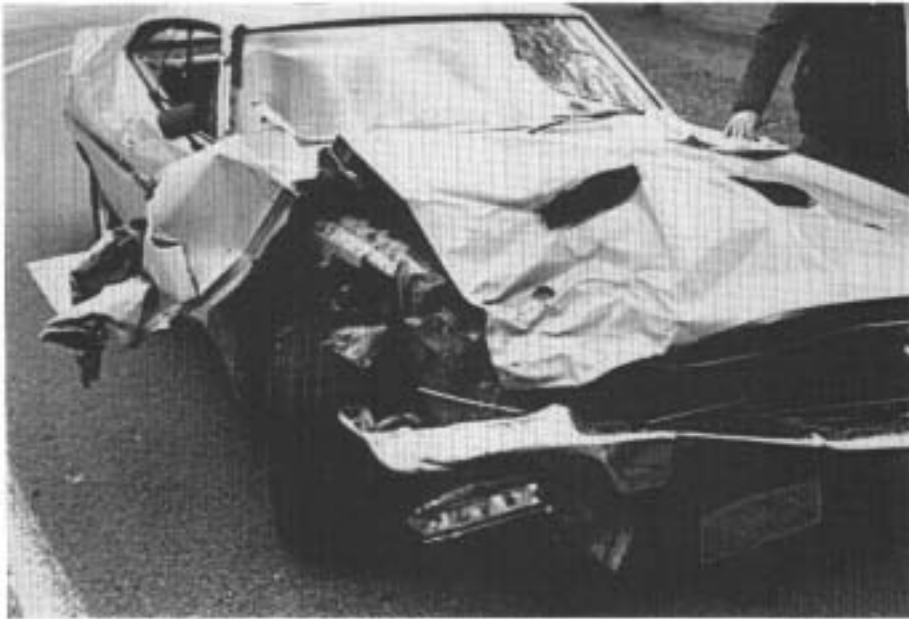
FIGURE A27: Crash 26. Impact damage to the right front and side of Ford Falcon.
