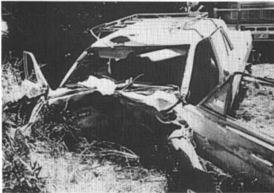
FIGURE A41: Crash 36. The passenger compartment of the car in its final position. The engine compartment, which separated in the second impact with a tree, came to rest in the trees behind the passenger compartment.
