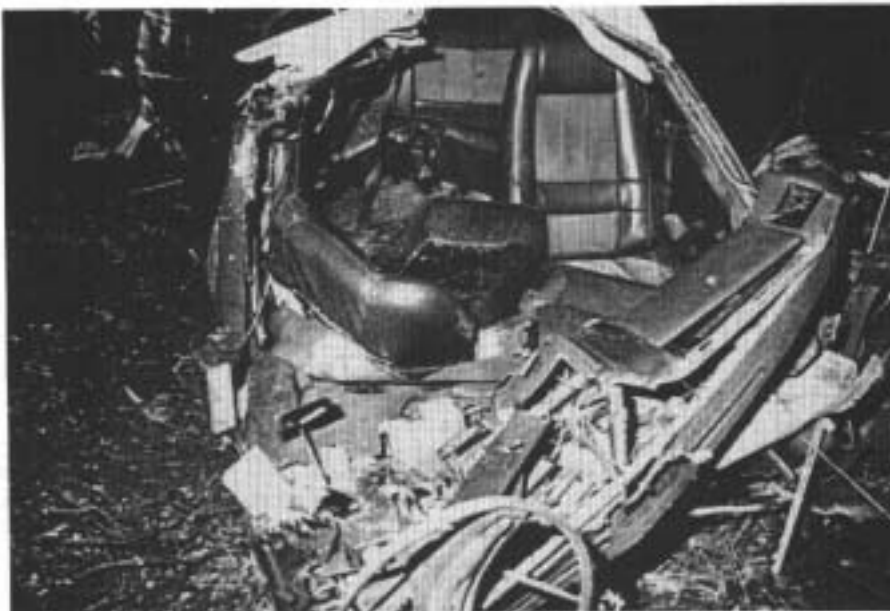
FIGURE A4: Crash 04. Damage to Ford Falcon stationwagon following impact with tree. The front of the car has been torn off exposing the passenger compartment. Note that the driver's seat is detached from its mounting.
