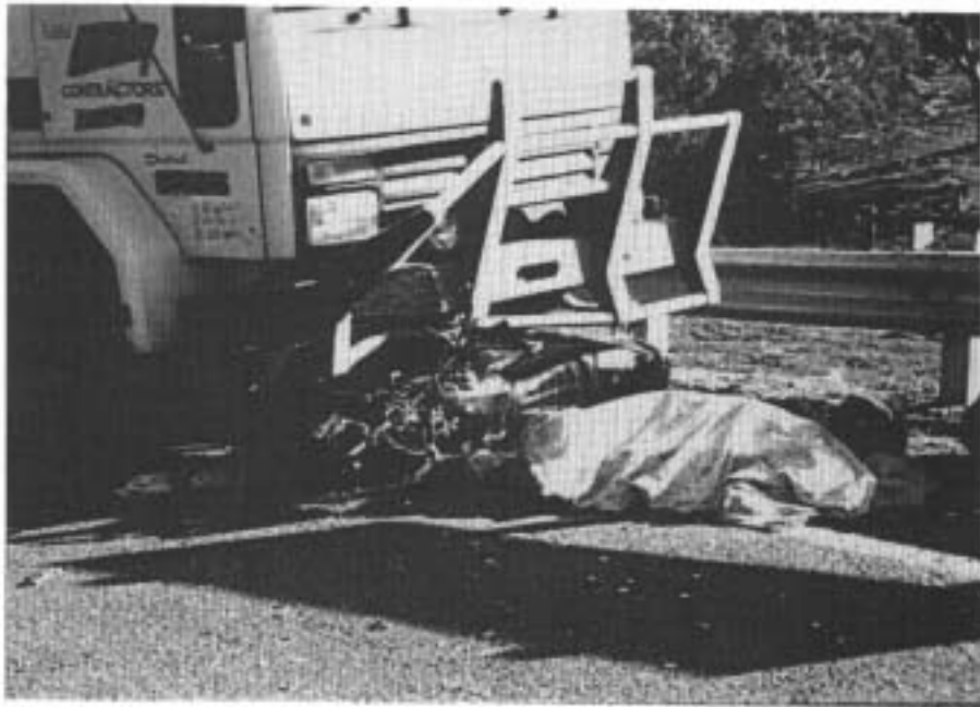
FIGURE A5: Crash 05. Final positions of motorcycle and dump truck. The motorcycle came to rest wedged under the front of the dump truck.
