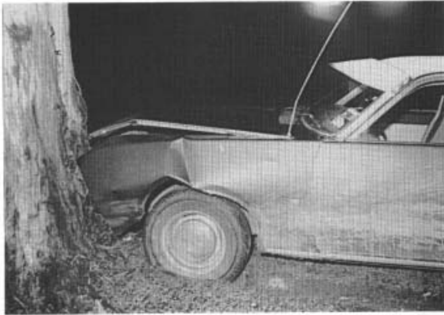
FIGURE A11: Crash 11. Impact damage to the left side of the car. Note deflated left front tyre.
