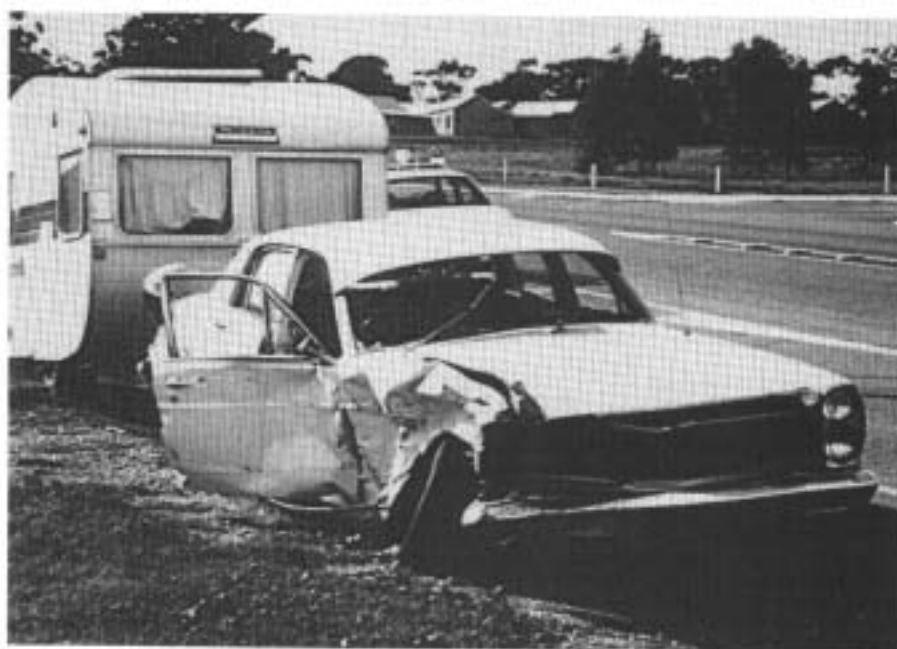
FIGURE A2: Crash 02. Ford Fairlane and caravan in rest position showing impact damage to right side.
