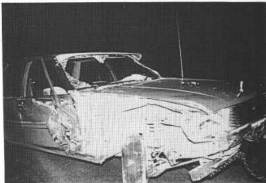
FIGURE A28: Crash 27. Impact damage to the right side of Ford Falcon. Note shattered windscreen, struck by front seat passenger.
