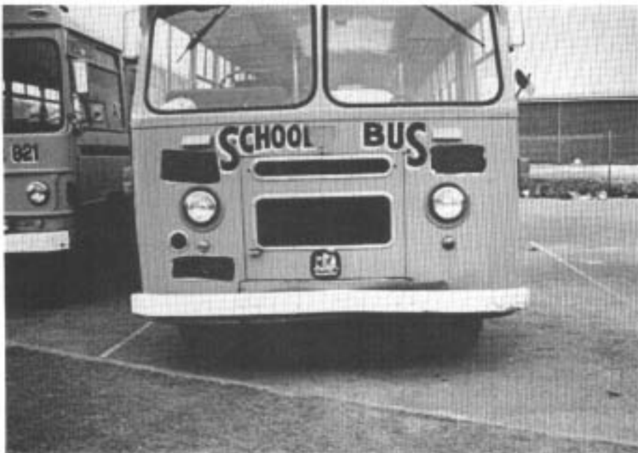
FIGURE A34: Crash 30. School bus. Damage above left end of bumper bar due to contact with motorcycle, which was on its left side.
