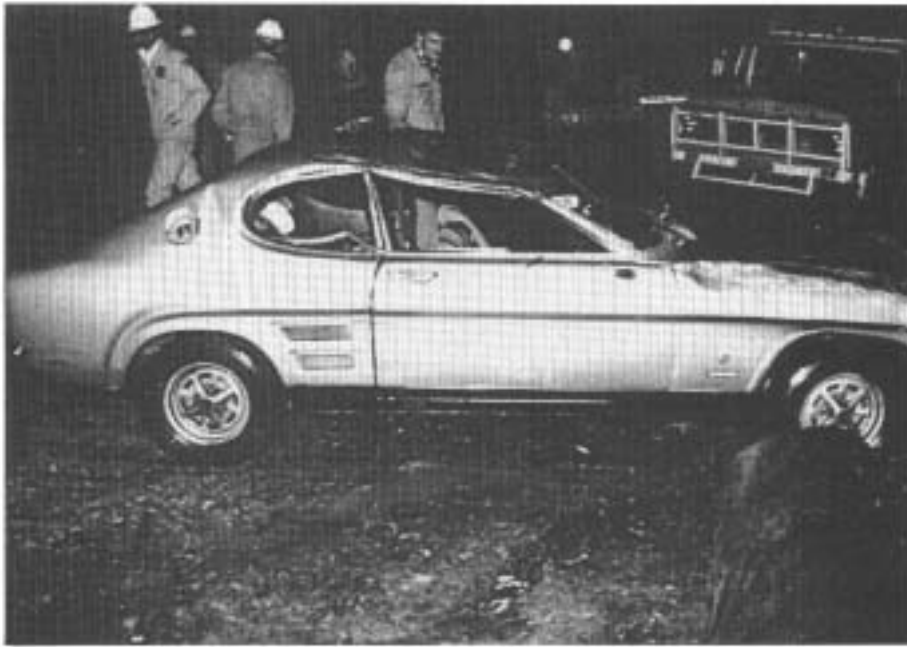
FIGURE A17: Crash 17. Ford Capri after being righted showing distortion of roof resulting from rollover, and scrape marks on the right front mudguard from contacting the road surface.
