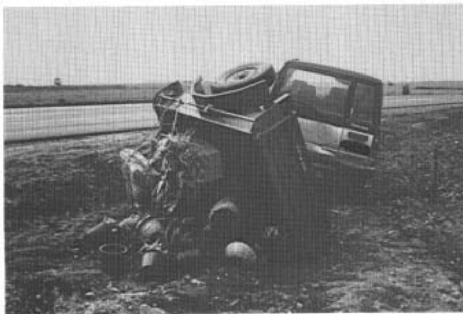
FIGURE A22: Crash 21. The final position of the Holden Jackaroo which came to rest on its left side and has been rolled back onto its wheels.
