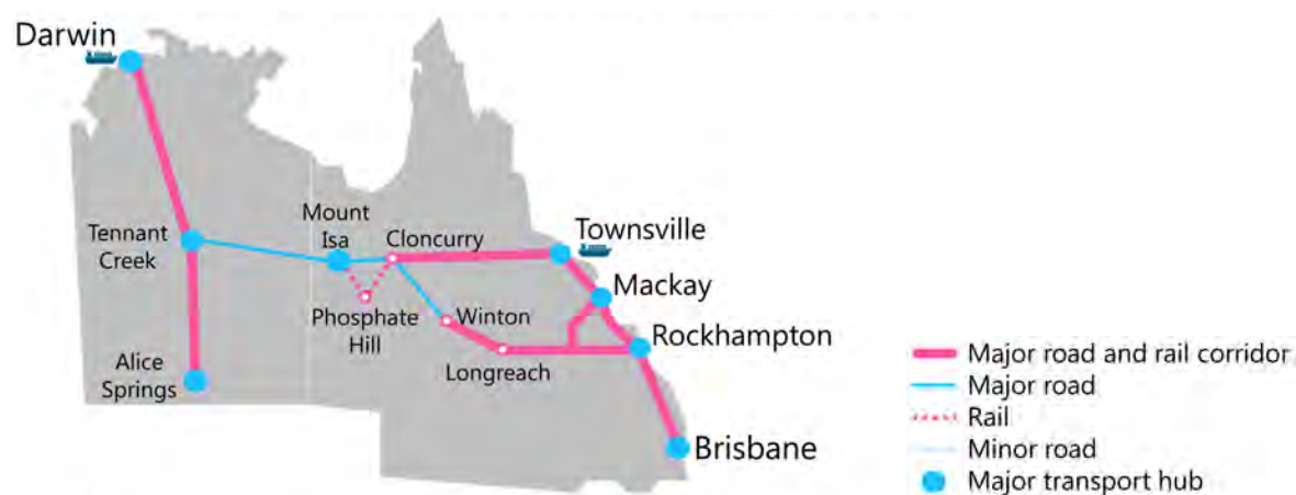
Figure 3.23: The current operation of the Darwin to Townsville supply chain, transporting between 3 to 5 mtpa between Darwin and Mount Isa, and approximately 7 mtpa between Mount Isa and Townsville
