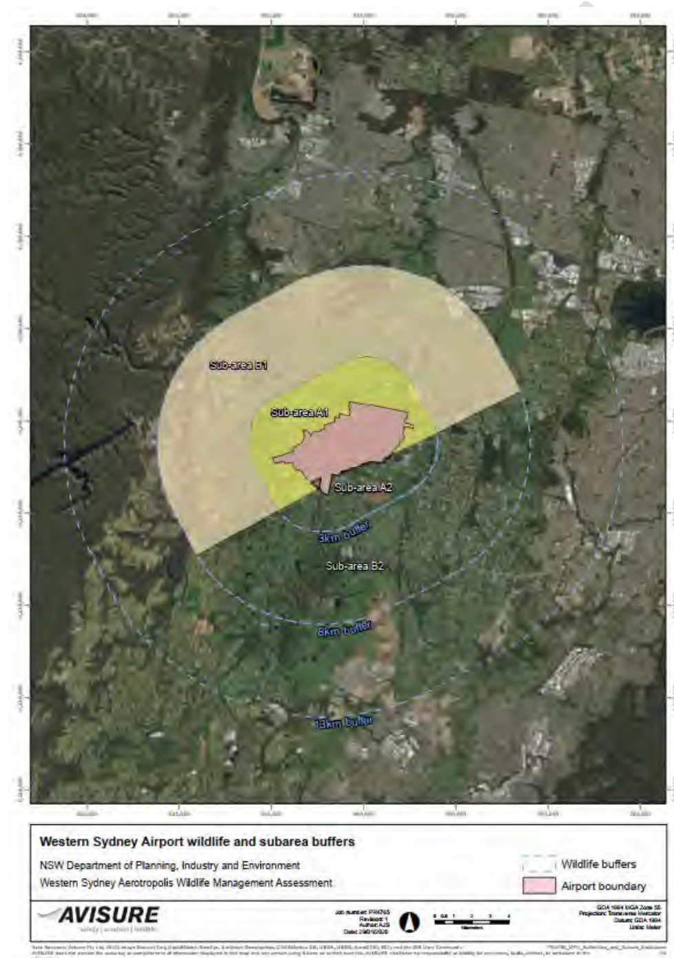
Figure 2. Area shaded red (sub-area A1) in 3km buffer requires more scrutiny (above NASF recommendation) to minimise wildlife crossing the airport to access food/water sources. Aims to reduce wildlife crossing from south-east to north west. Area shaded orange (sub-area B1) in 8km buffer requires more scrutiny (above NASF recommendation), but not as rigid as the 3km buffer red zone, to minimise wildlife crossing the airport to access food/water sources.
