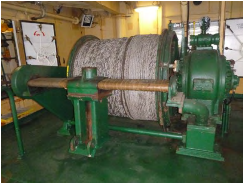
Port Trawl winch with 3927 meters of 22mm RHOL wire
