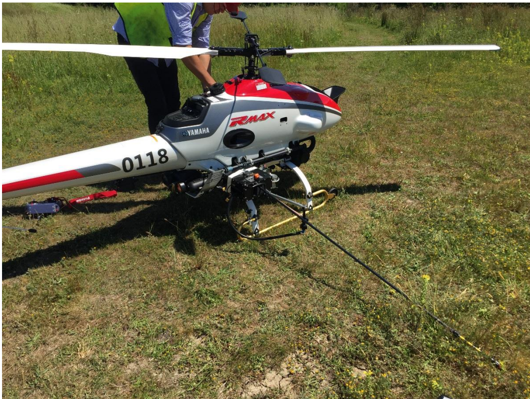
Figure 8. Spray lance attached to Australia's only agriculturally-certified drone. Note this photograph is of the R-max which has now been superseded by the Fazer.
