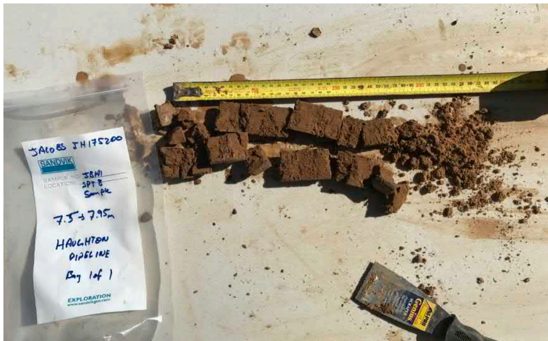
Photograph 8 - JBH1 SPT Sample from 7.5 - 7.95m.
