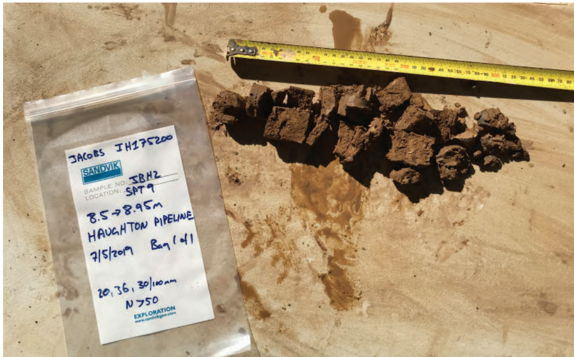
Photograph 29 - JBH2 SPT Sample from 8.5 - 8.95m.
