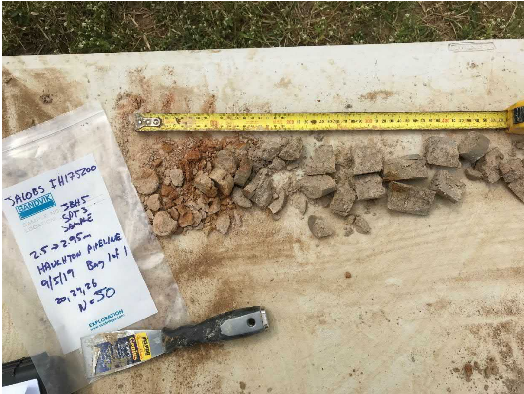
Photograph 68 – JBH5 SPT Sample from 2.5 -2.95m.
