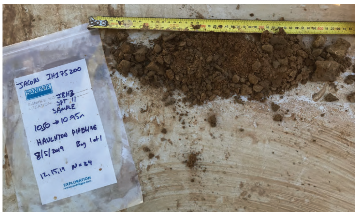
Photograph 43 - JBH3 SPT Sample from 10.5 - 10.95m.
