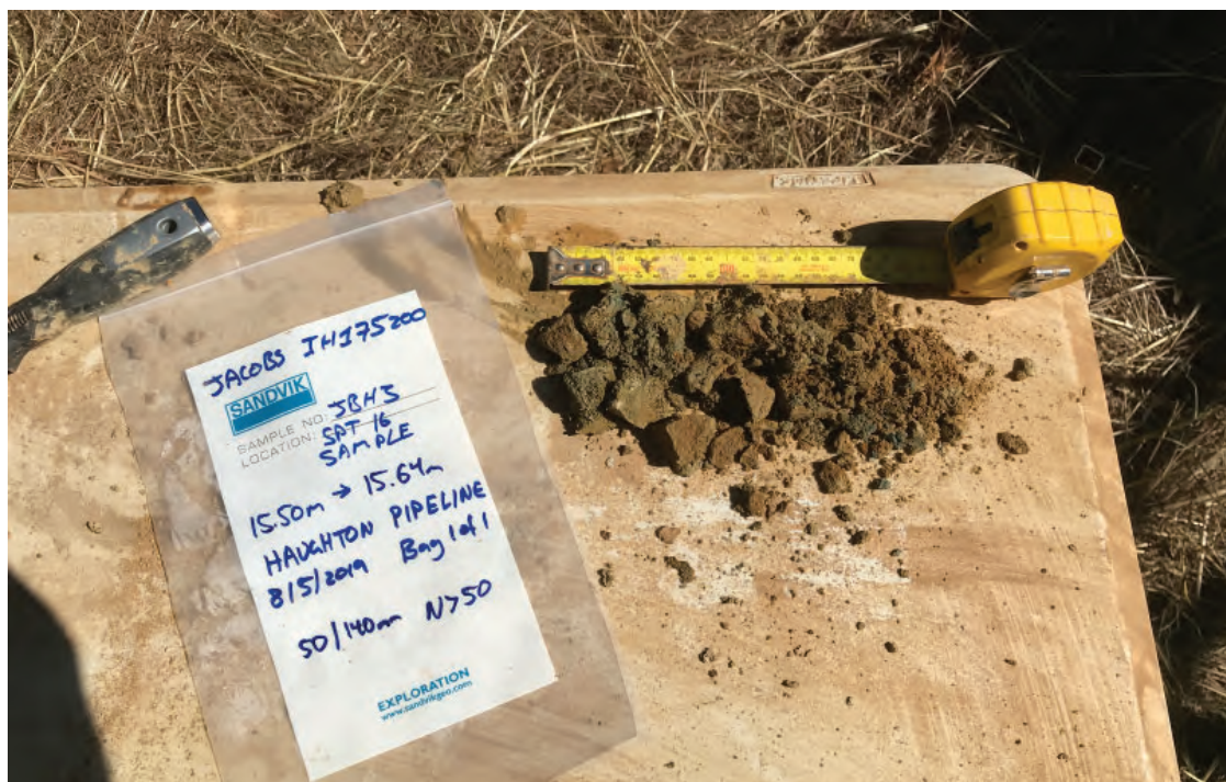
Photograph 48 - JBH3 SPT Sample from 15.5 - 15.67m.
