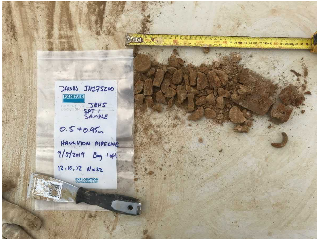
Photograph 66 – JBH5 SPT Sample from 0.5 -0.95m.
