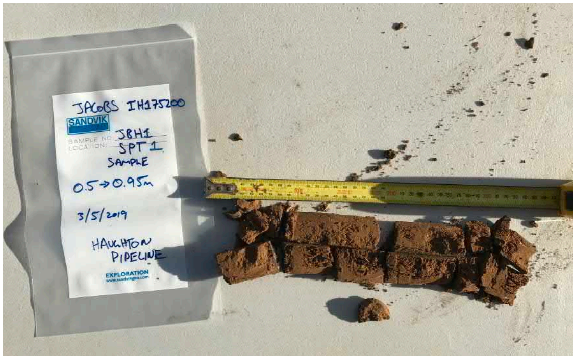
Photograph 3 - JBH1 SPT Sample from 0.5 - 0.95m.
