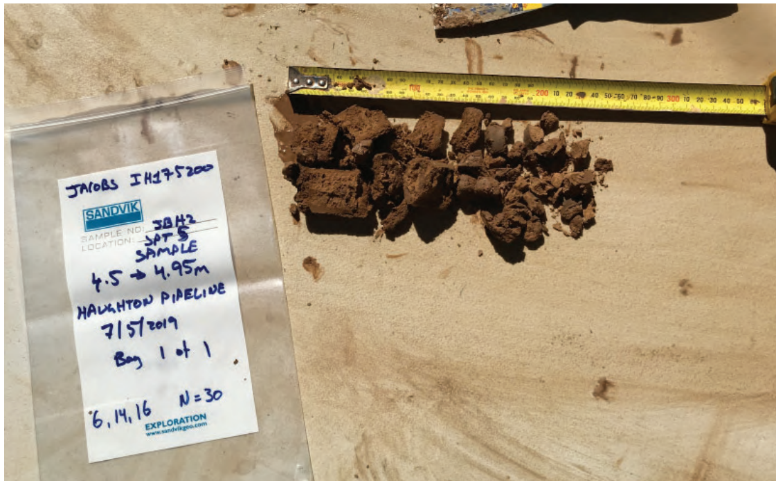
Photograph 25 - JBH2 SPT Sample from 4.5 - 4.95m.
