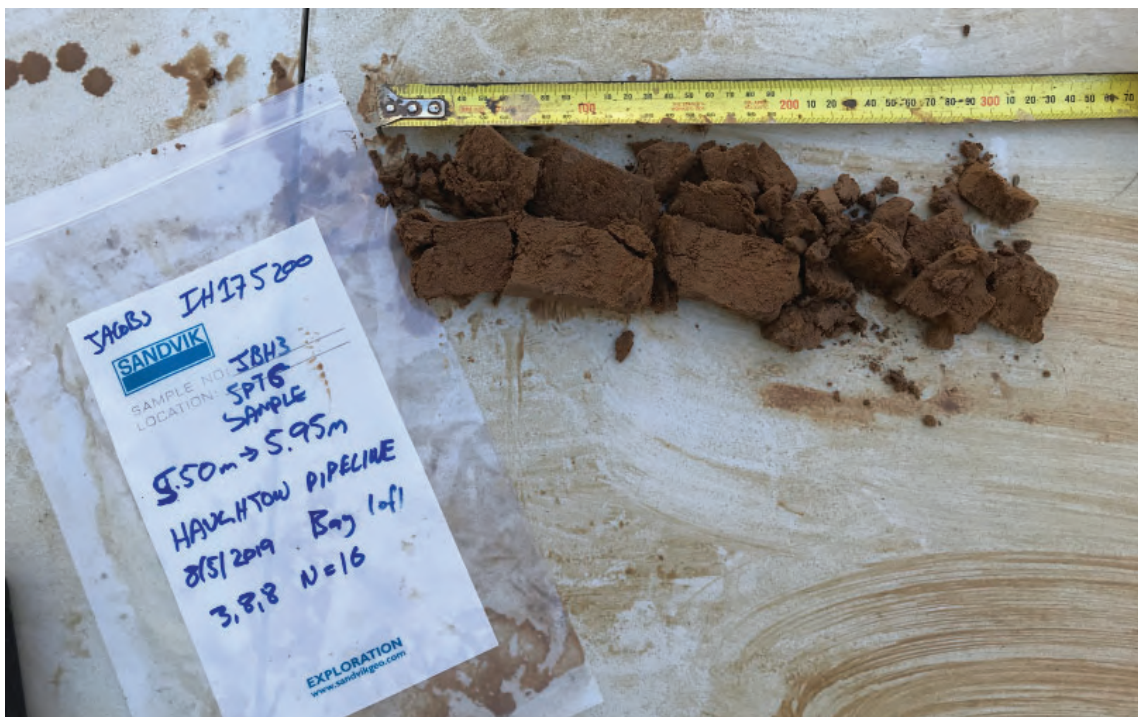
Photograph 38 - JBH3 SPT Sample from 5.5 - 5.95m.
