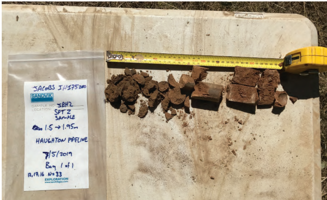
Photograph 22 - JBH2 SPT Sample from 1.5 - 1.95m.
