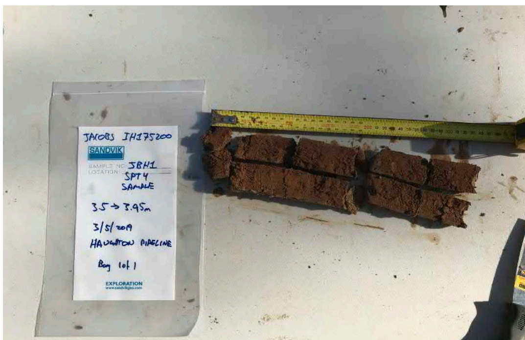
Photograph 6 - JBH1 SPT Sample from 3.5 - 3.95m.
