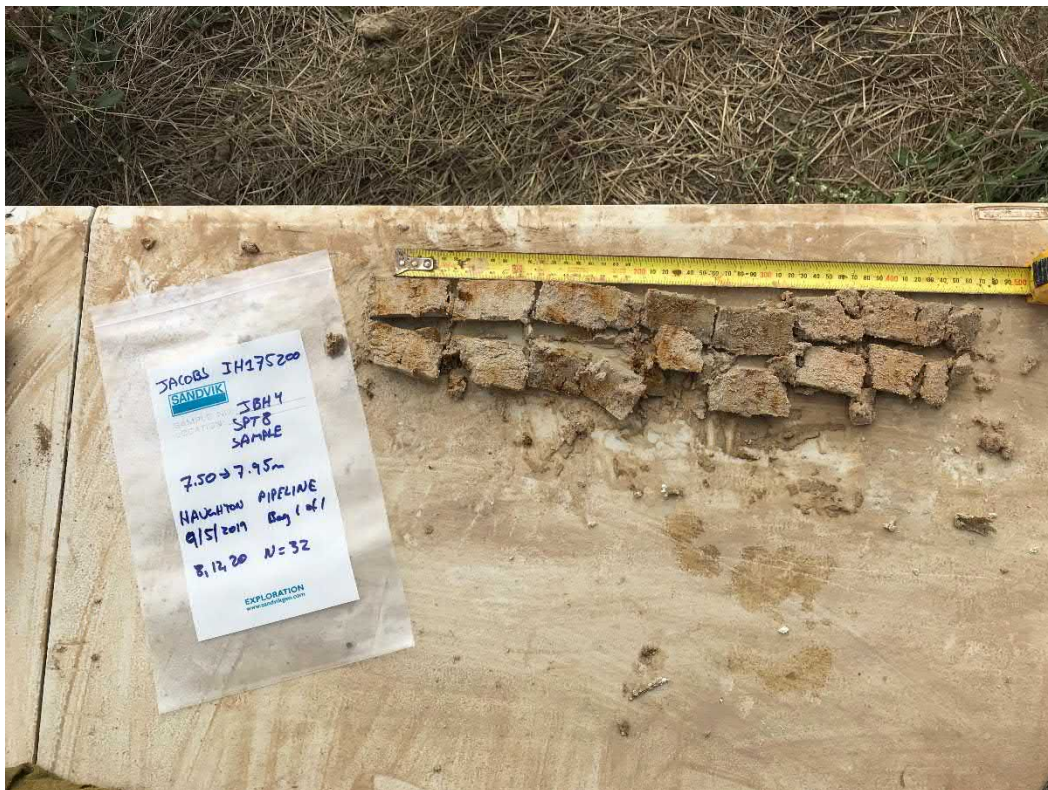
Photograph 61 – JBH4 SPT Sample from 7.5 - 7.95m.
