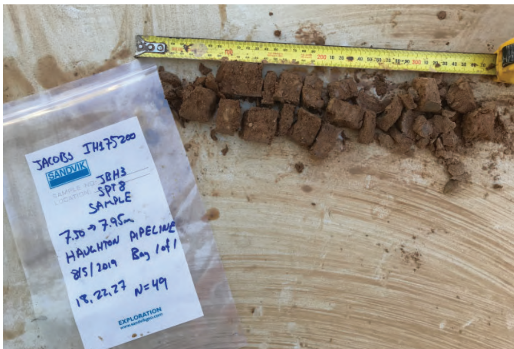
Photograph 40 - JBH3 SPT Sample from 7.5 - 7.95m.
