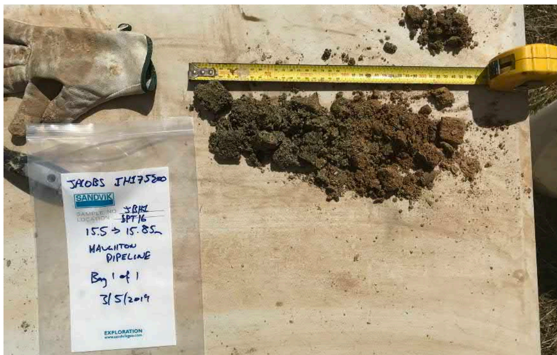
Photograph 15 - BH1 SPT Sample from 15.5 - 15.85m.
