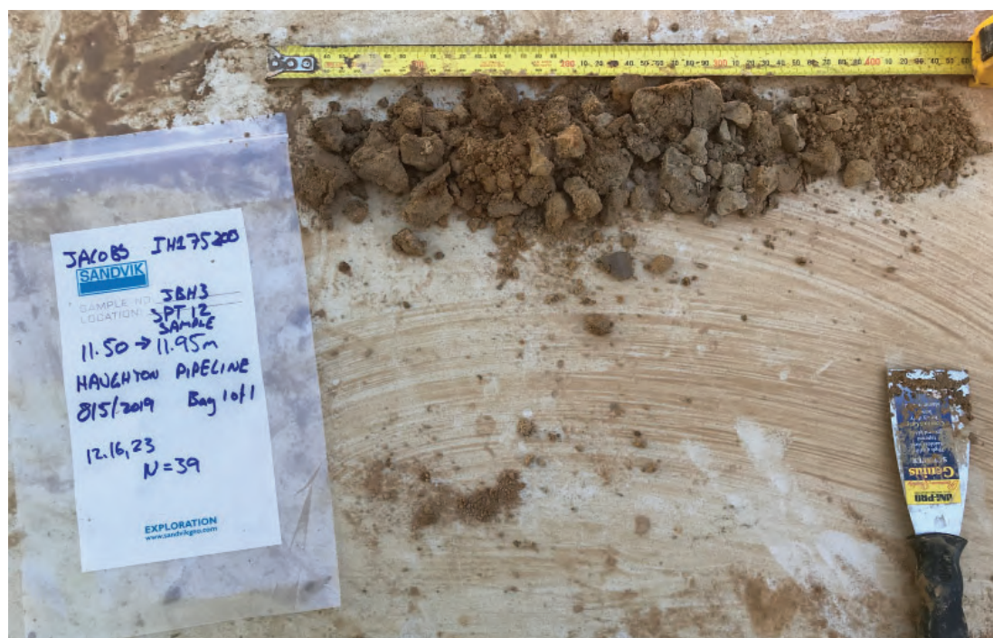
Photograph 44 - JBH3 SPT Sample from 11.5 - 11.95m.
