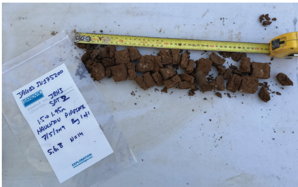
Photograph 34 - JBH3 SPT Sample from 1.5 - 1.95m.
