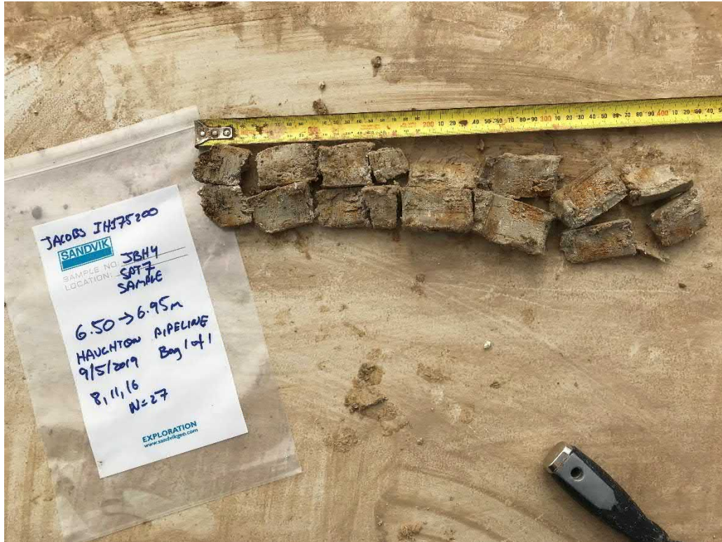
Photograph 60 – JBH4 SPT Sample from 6.5 - 6.95m.
