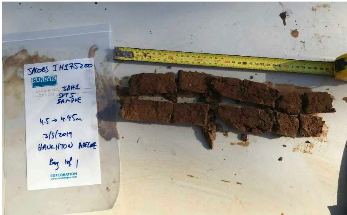
Photograph 7 - JBH1 SPT Sample from 4.5 - 4.95m.
