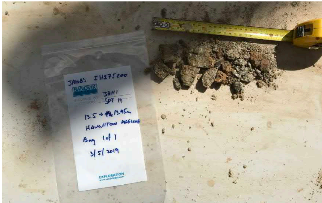
Photograph 13 JBH1 SPT Sample from 13.5 - 13.95m
