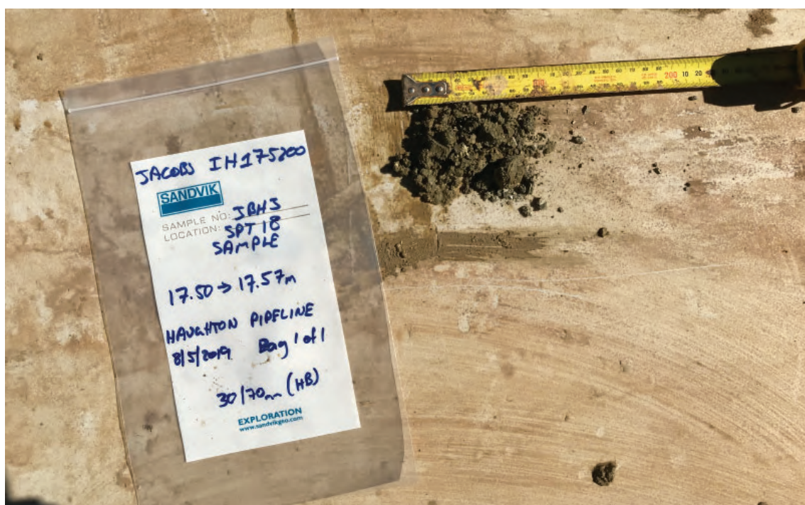
Photograph 50 - JBH3 SPT Sample from 17.5 - 17.57m.
