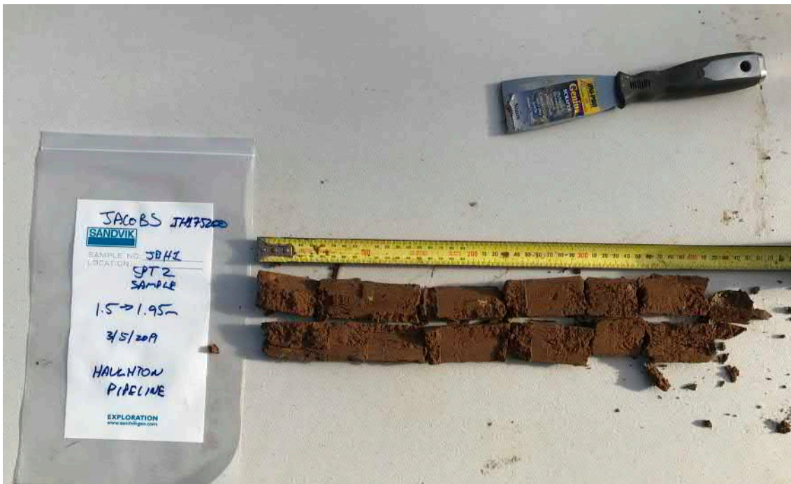
Photograph 4 - JBH1 SPT Sample from 1.5 - 1.95m.
