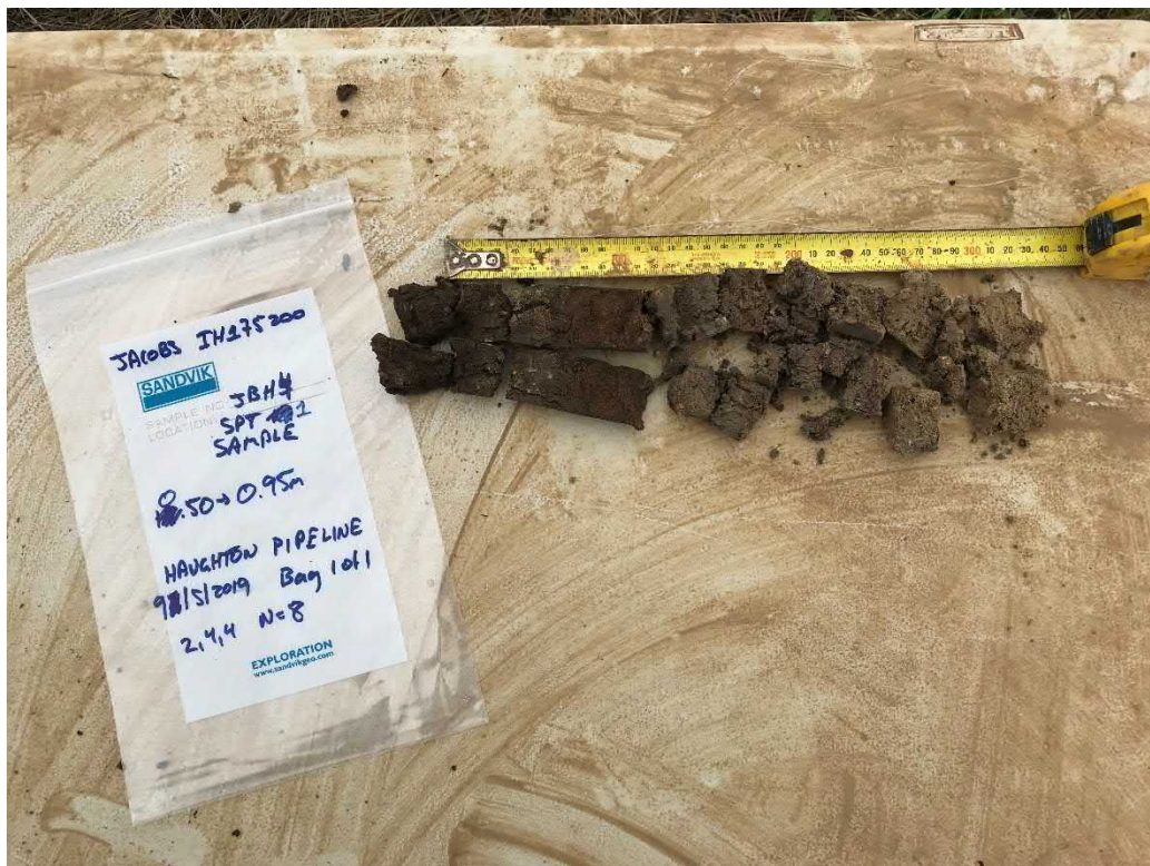
Photograph 54 – JBH4 SPT Sample from 0.5 - 0.95m.
