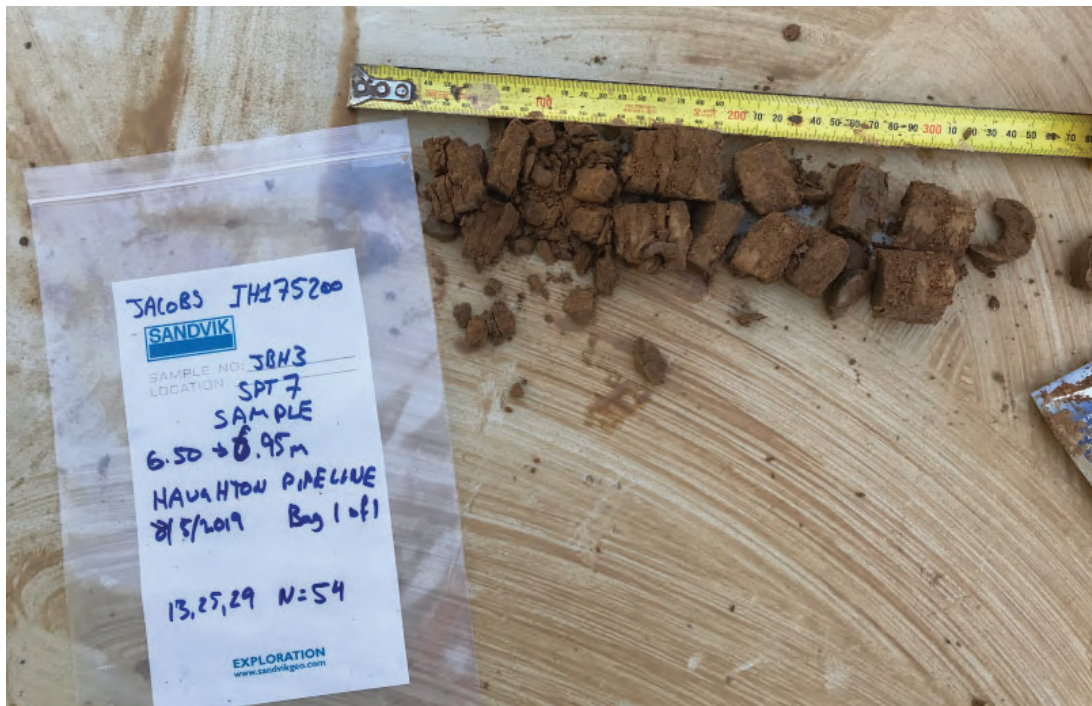
Photograph 39 - JBH3 SPT Sample from 6.5 - 6.95m.
