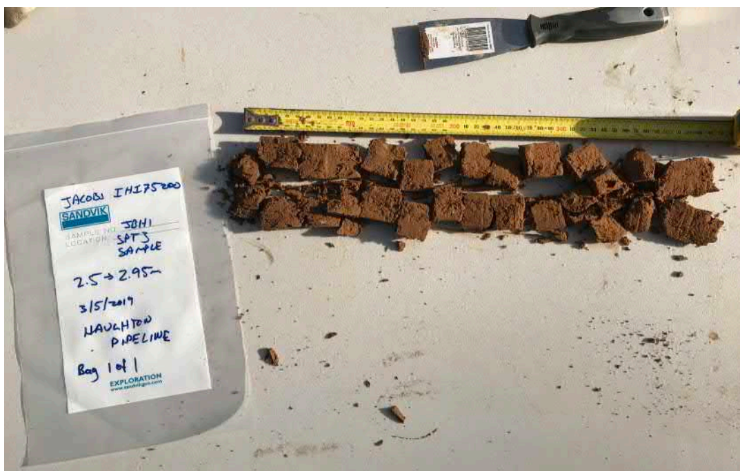
Photograph 5 - JBH1 SPT Sample from 2.5 - 2.95m.
