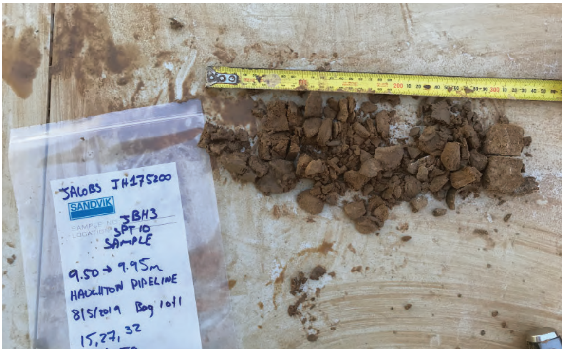
Photograph 42 - JBH3 SPT Sample from 9.5 - 9.95m.
