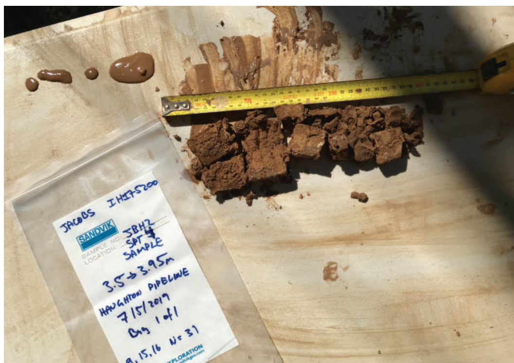
Photograph 24 - JBH2 SPT Sample from 3.5 - 3.95m.
