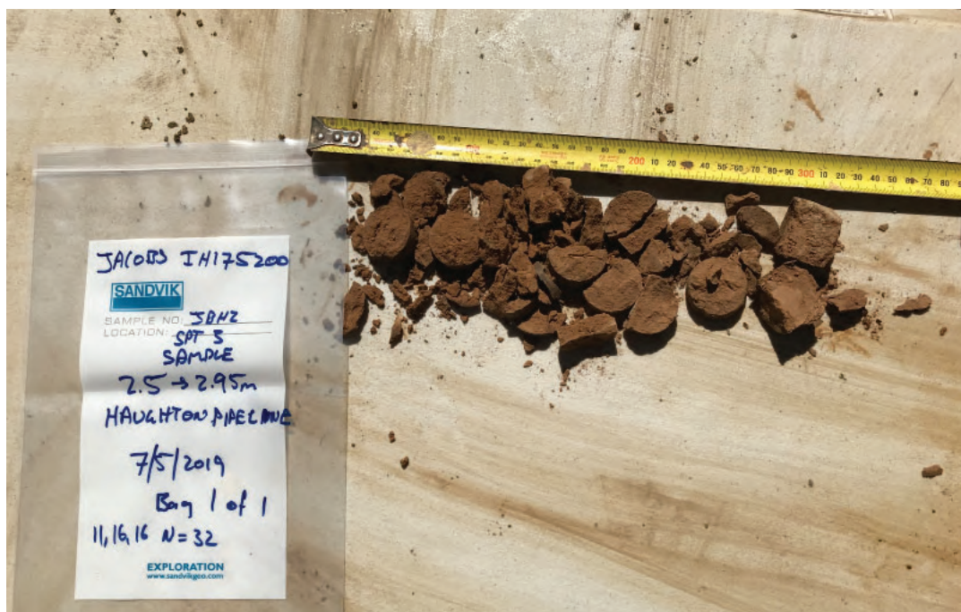
Photograph 23 - JBH2 SPT Sample from 2.5 - 2.95m.
