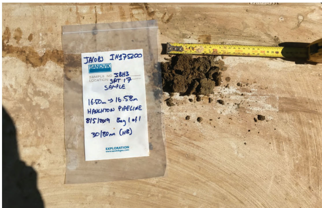
Photograph 49 - JBH3 SPT Sample from 16.5 - 16.58m.
