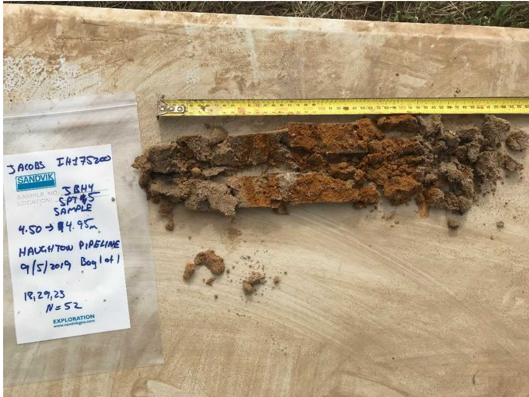
Photograph 58 – JBH4 SPT Sample from 4.5 - 4.95m.
