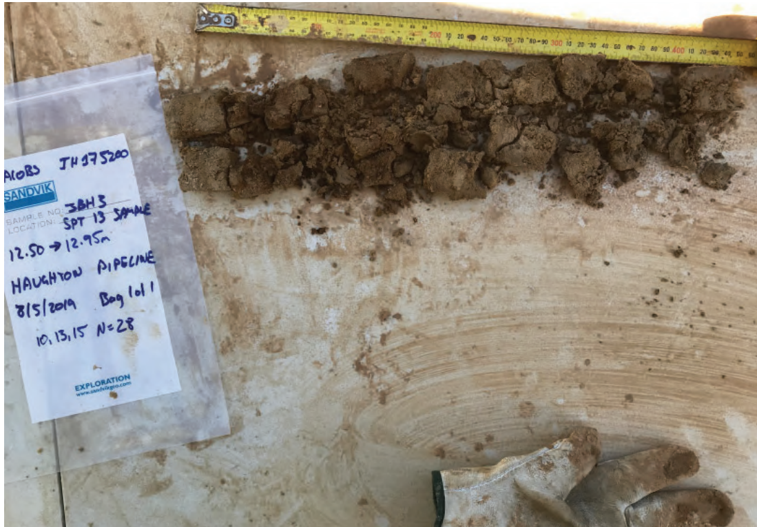
Photograph 45 - JBH3 SPT Sample from 12.5 - 12.95m.
