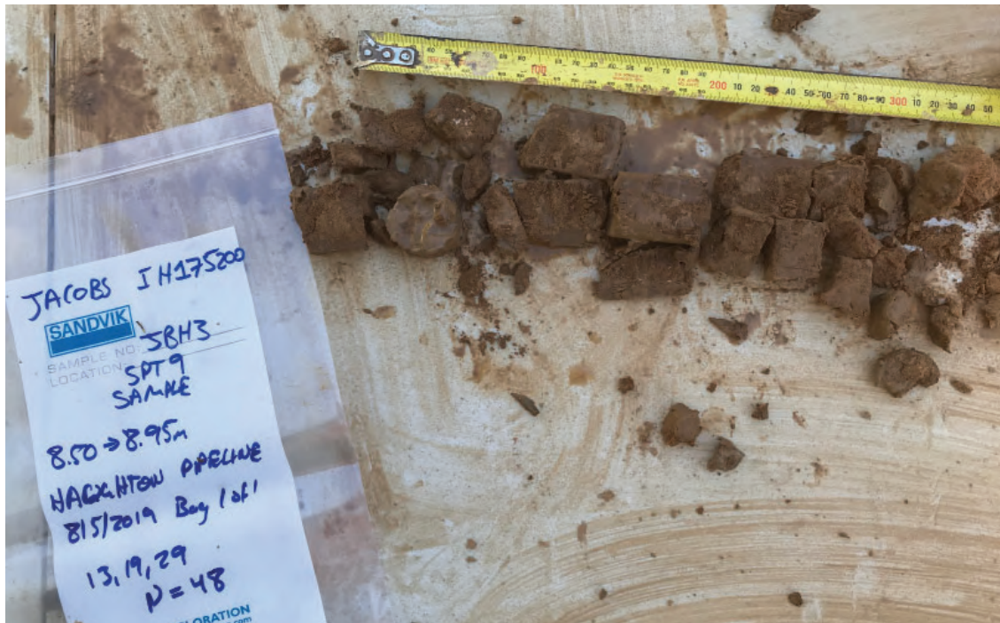
Photograph 41 - JBH3 SPT Sample from 8.5 - 8.95m.
