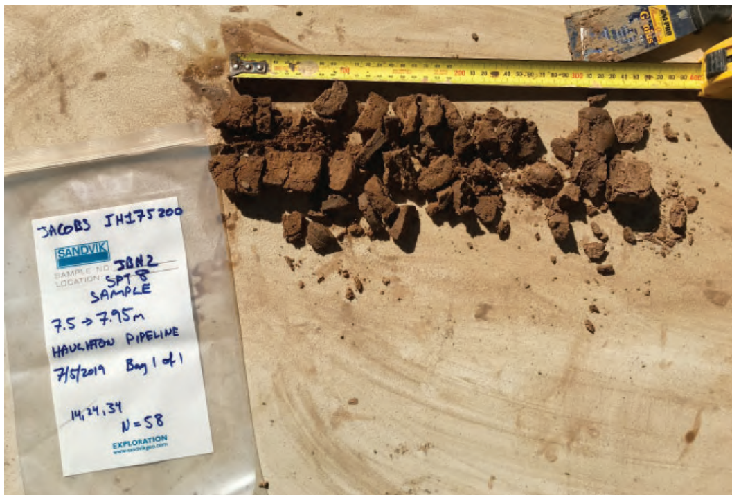
Photograph 28 - JBH2 SPT Sample from 7.5 - 7.95m.
