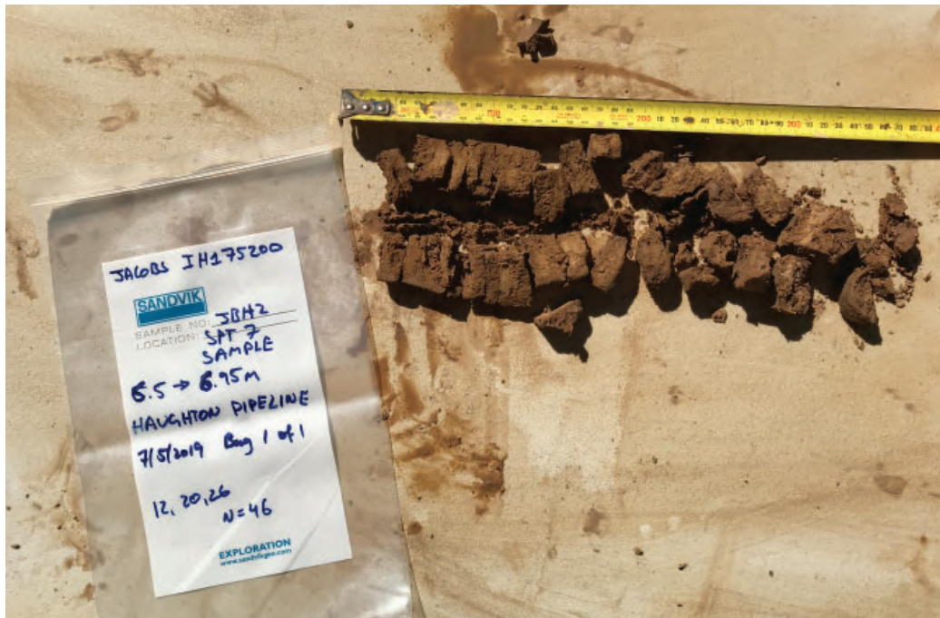
Photograph 27 - JBH2 SPT Sample from 6.5 - 6.95m.
