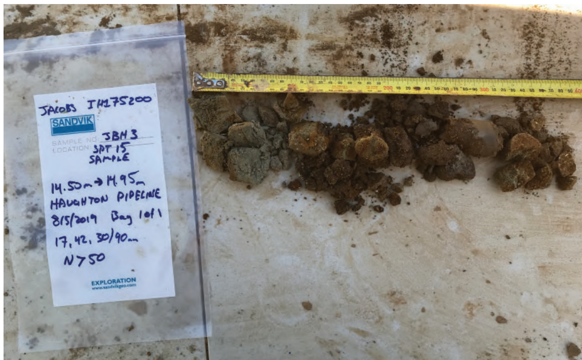
Photograph 47 - JBH3 SPT Sample from 14.5 - 14.85m.
