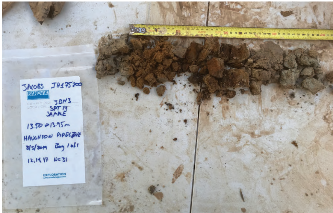
Photograph 46 - JBH3 SPT Sample from 13.5 - 13.95m.
