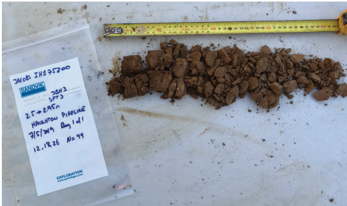
Photograph 35 - JBH3 SPT Sample from 2.5 - 2.95m.
