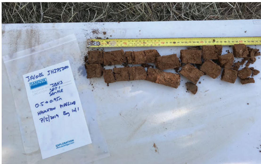
Photograph 33 - JBH3 SPT Sample from 0.5 - 0.95m.
