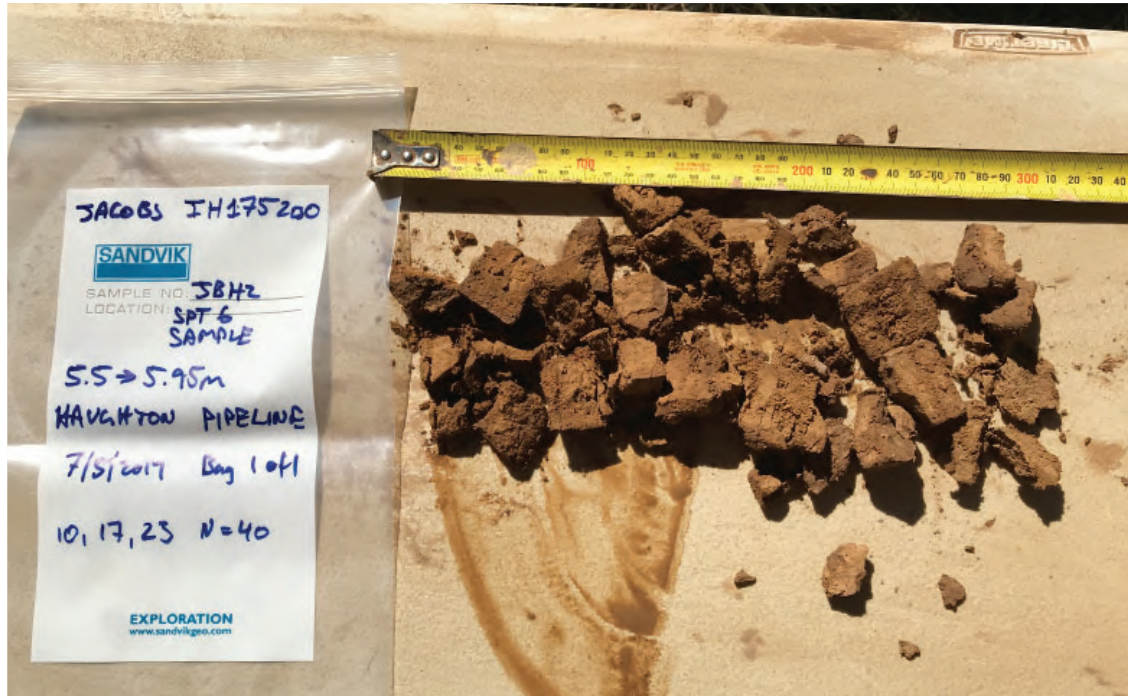
Photograph 26 - JBH2 SPT Sample from 5.5 - 5.95m.
