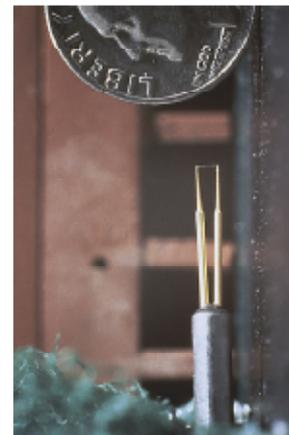
One of the advantages of hot wires is that they can be mounted at the ends of probes which can be positioned to measure wind speeds at any location of interest, eg to identify the extent of the wake behind a building at any height above ground level.
