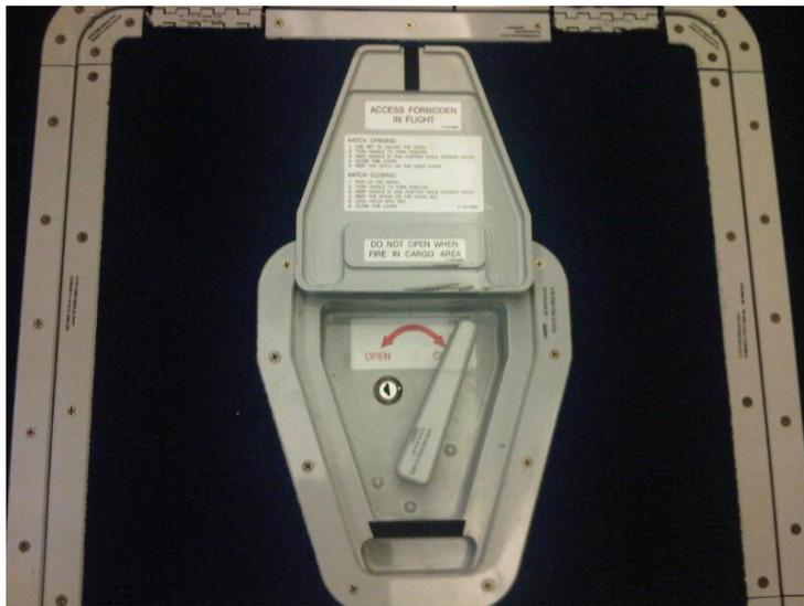
*Fig 7. Airbus Hatch For Aft Cabin Flooring - locking handle in view (KC30 RAAF).*
