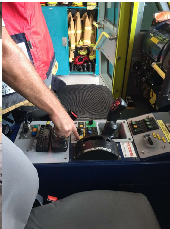
Photo 64. Foam switch location in the fire tender located near the gear stick.
