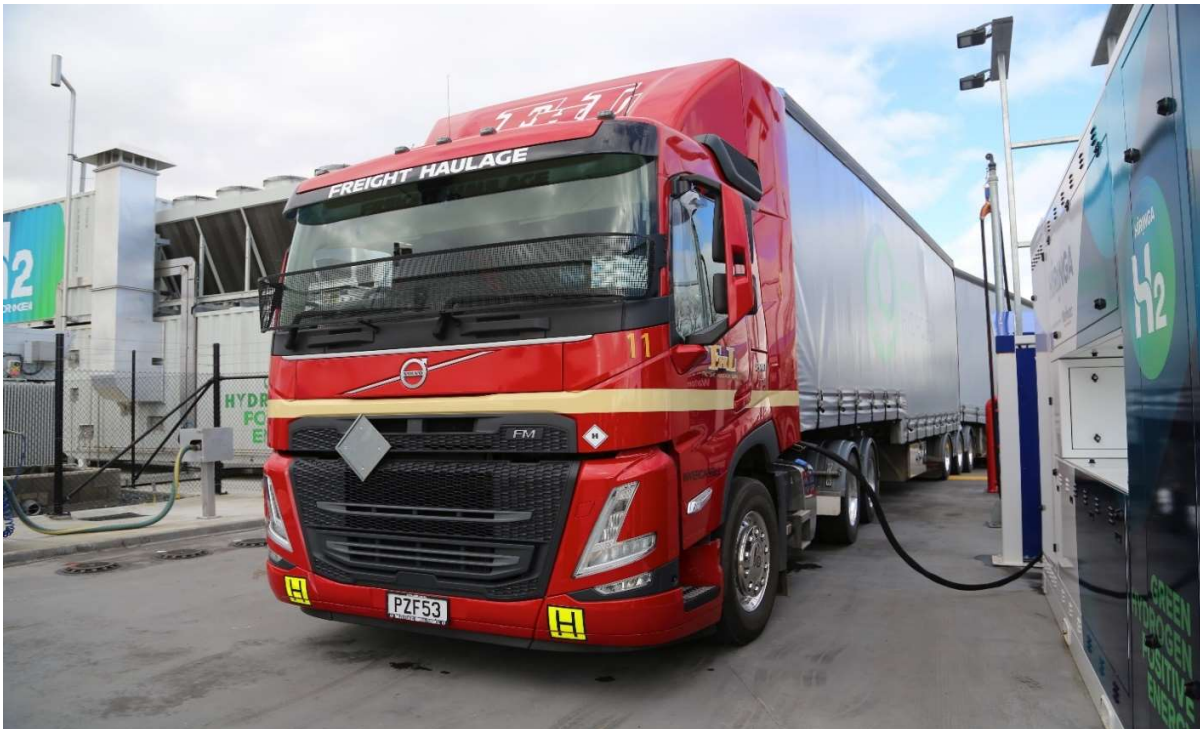
Picture courtesy of NZ Trucking Media: MyTransport's dual fuel integrated into Volvo FM Prime Mover (30kg hydrogen storage) with B-Double trailer fueling with H2 at Hiringa Auckland station
