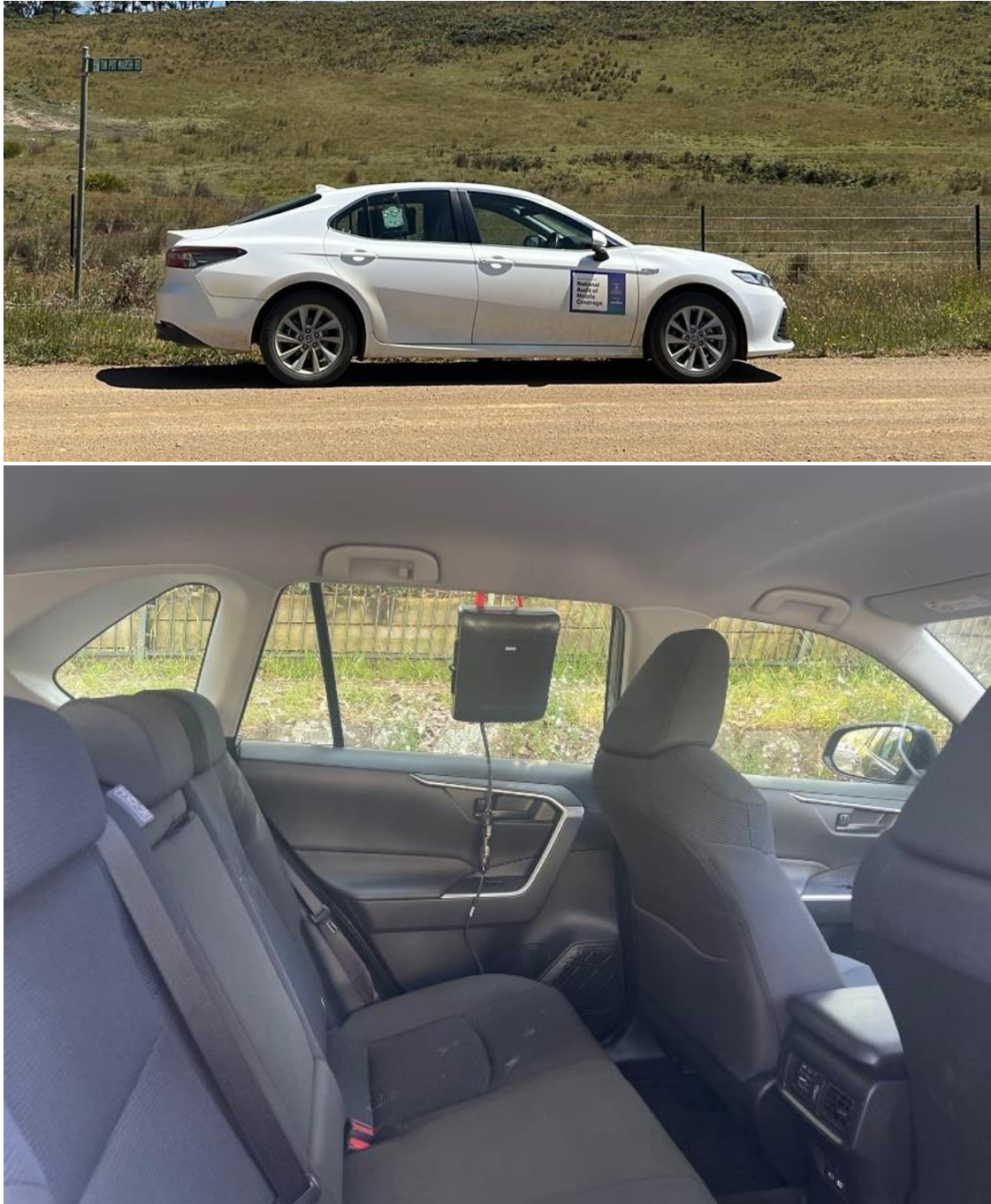
Figure 3: Typical Audit Roads setup for Accenture vehicles, with window-mounted testing kits.
