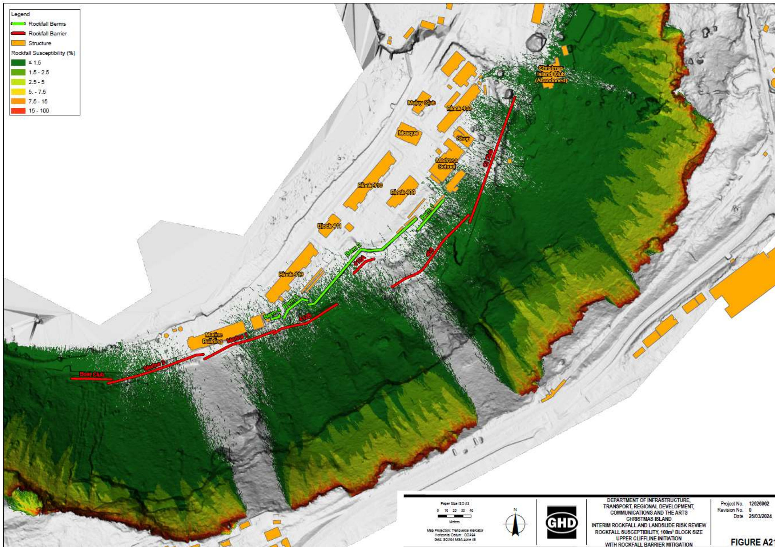
FIGURE 2 – Rockfall Susceptibility, 100 m 3 Block, Upper Cliffline Initiation (With existing barriers)
