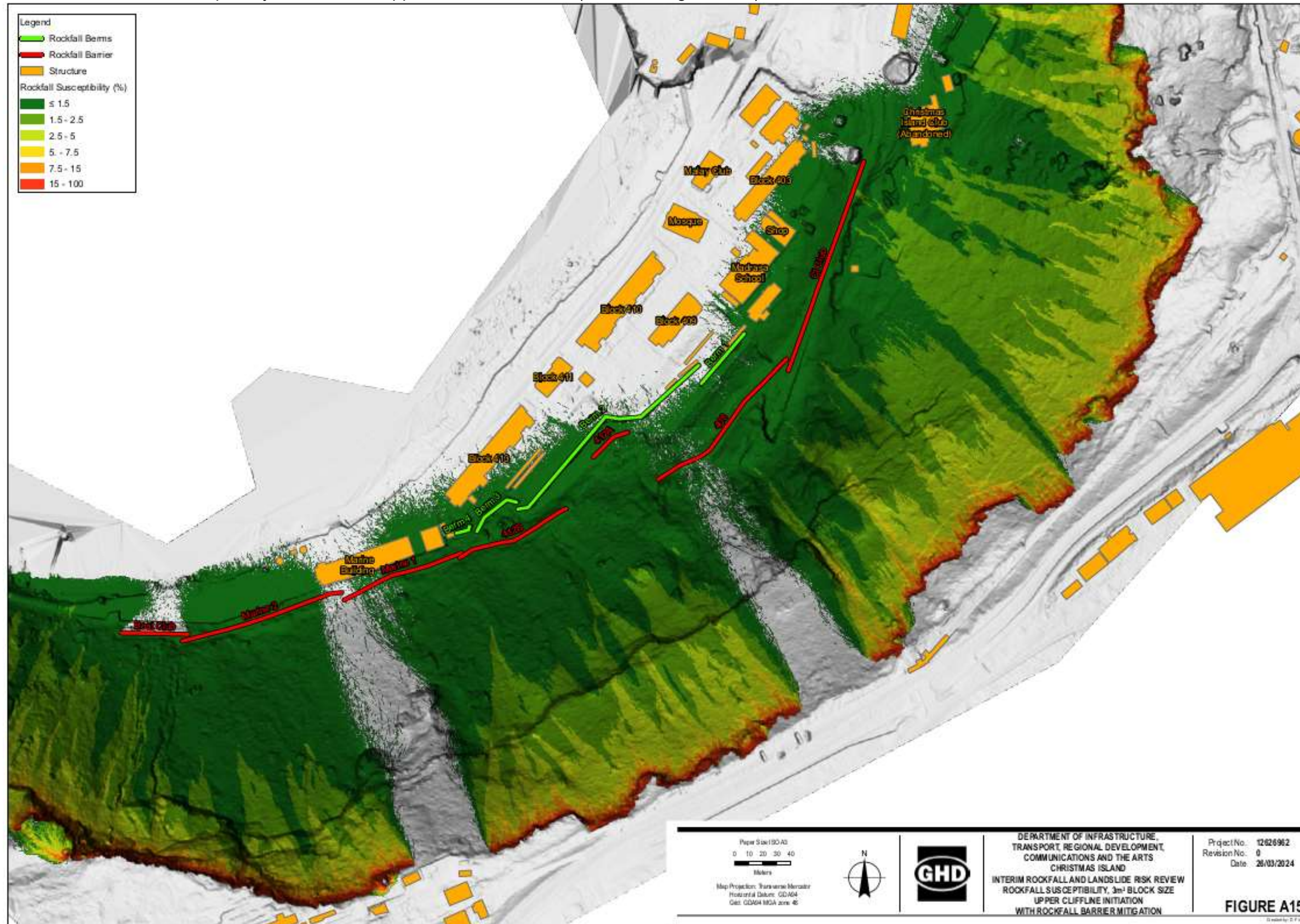
FIGURE 1 – Rockfall Susceptibility, 3 m³ Block, Upper Cliff line Initiation (With existing barriers)
