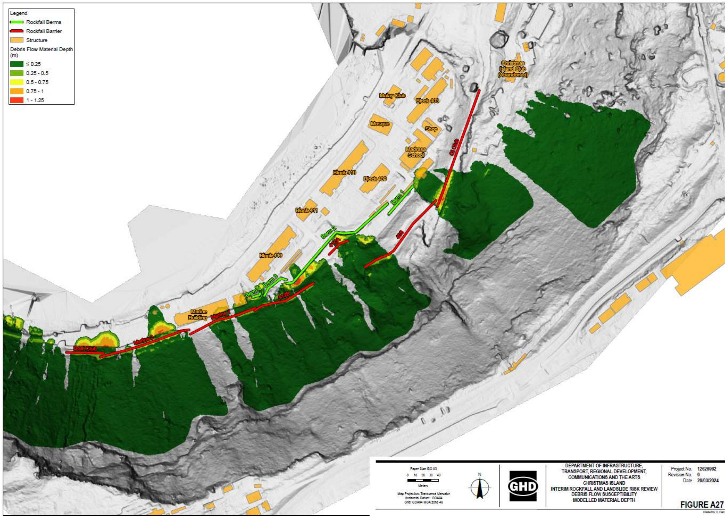
FIGURE 5 – Areas of Debris Flow Landslide Susceptibility
