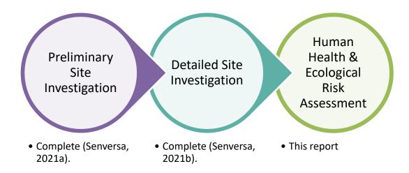
The Preliminary Site Investigation (PSI) and Detailed Site Investigation (DSI) identified PFAS sources, contaminant transport pathways and receptors potentially exposed to PFAS, and presented the findings of the initial, targeted investigation into the nature and extent of PFAS at the Norfolk Island Airport and surrounding catchments.
