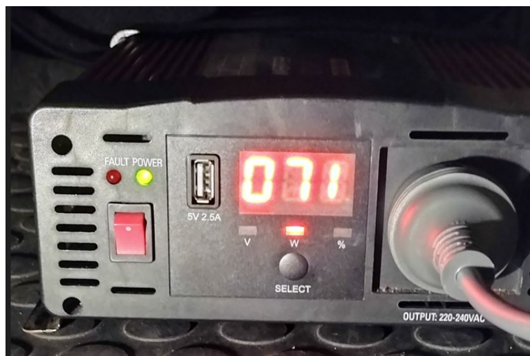
Figure 11: Maximum Starlink power draw (in Watts)
