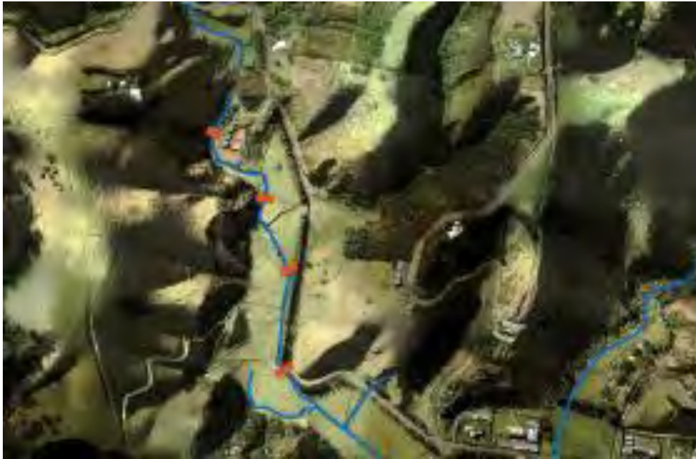
Figure 5: Leaky weir locations (Bligh Tanner, Figure 7, 2020)
