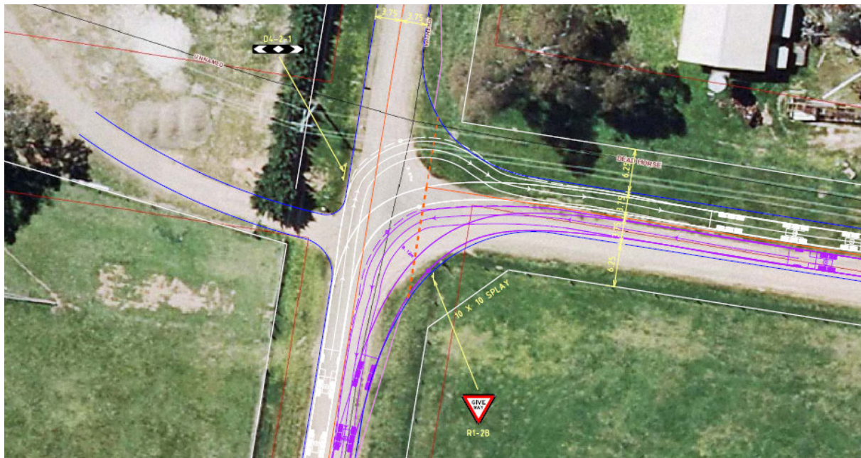
Figure 6.2.3a: Minimum Splay at Withers Lane/Dead Horse Lane intersection
