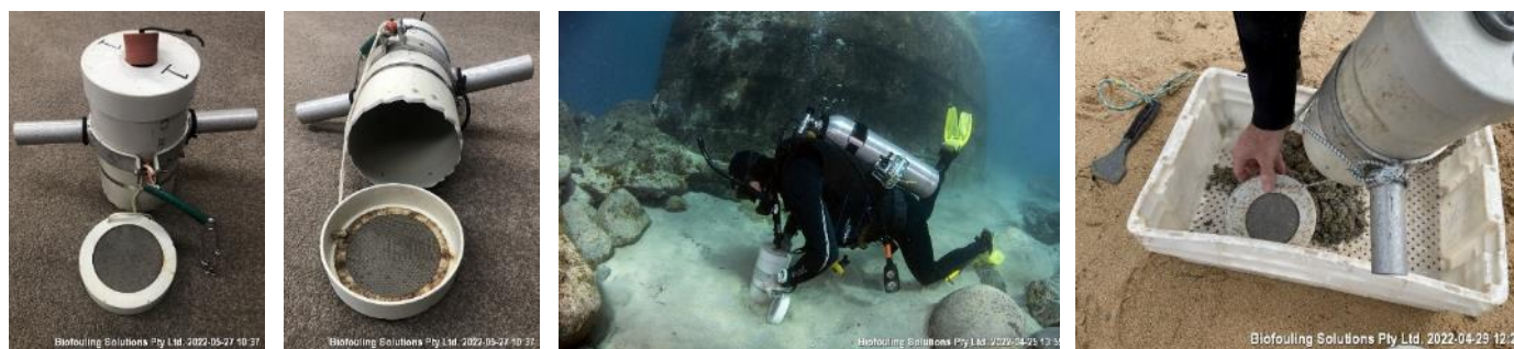
Figure 4. Benthic cores were used to sample soft sediments for potential IMS at Cascade Bay, Ball Bay, Emily Bay and Slaughter Bay.
