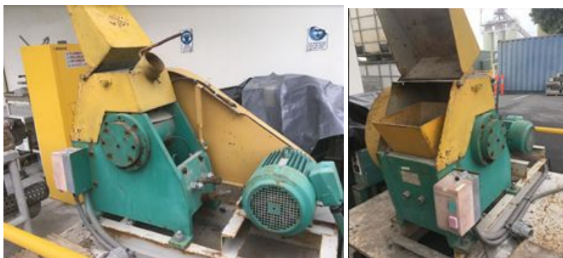
Figure 4 - Boral Whinstanes - Jaw Crusher
