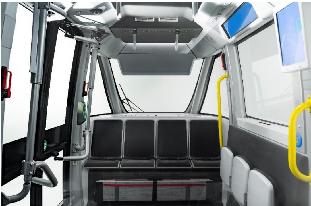
Figure 2. Interior of a typical shuttle (Navya) showing the seating arrangement, doors and handlebars.
