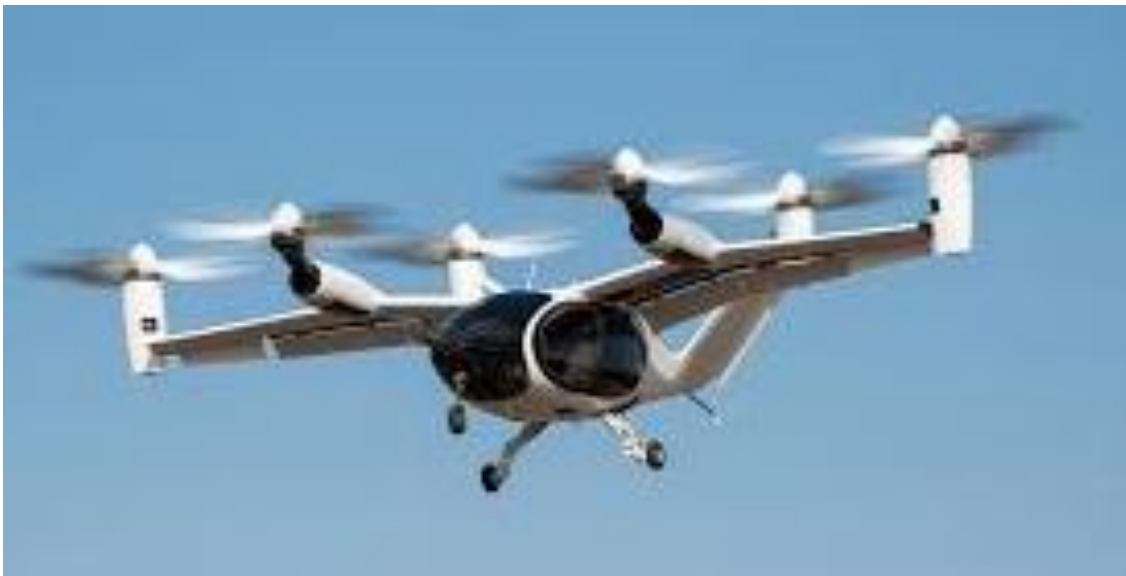
Figure 7. Joby S4 (The buyer of Uber elevate) has 6 propellers and wings.
