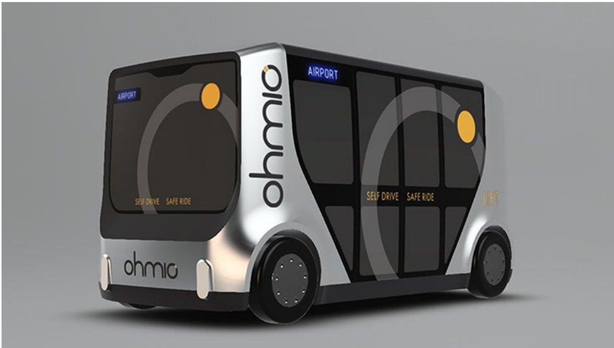
Figure 5. Exterior of a typical shuttle showing that the vehicle (Ohmio) has very small wheels, two large outward folding glass doors on the side and is mostly designed for standing passengers as there is a relatively large open floor space.
