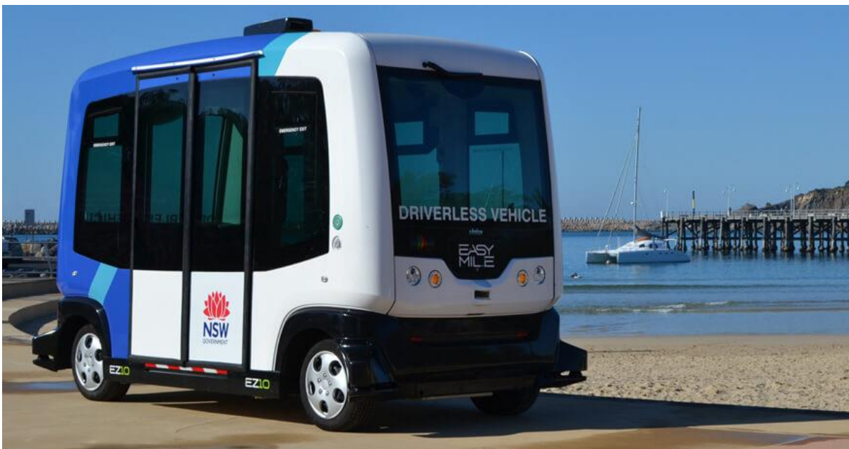
Figure 6. Exterior of a typical shuttle showing that the vehicle (Easymile) has very small wheels, two large outward folding glass doors on the side and is mostly designed for standing passengers as there is a relatively large open floor space.
