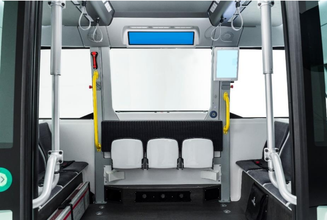
Figure 1. Interior of a typical shuttle (Navya) showing the seats at the front and rear end plus jump seats along the side.
