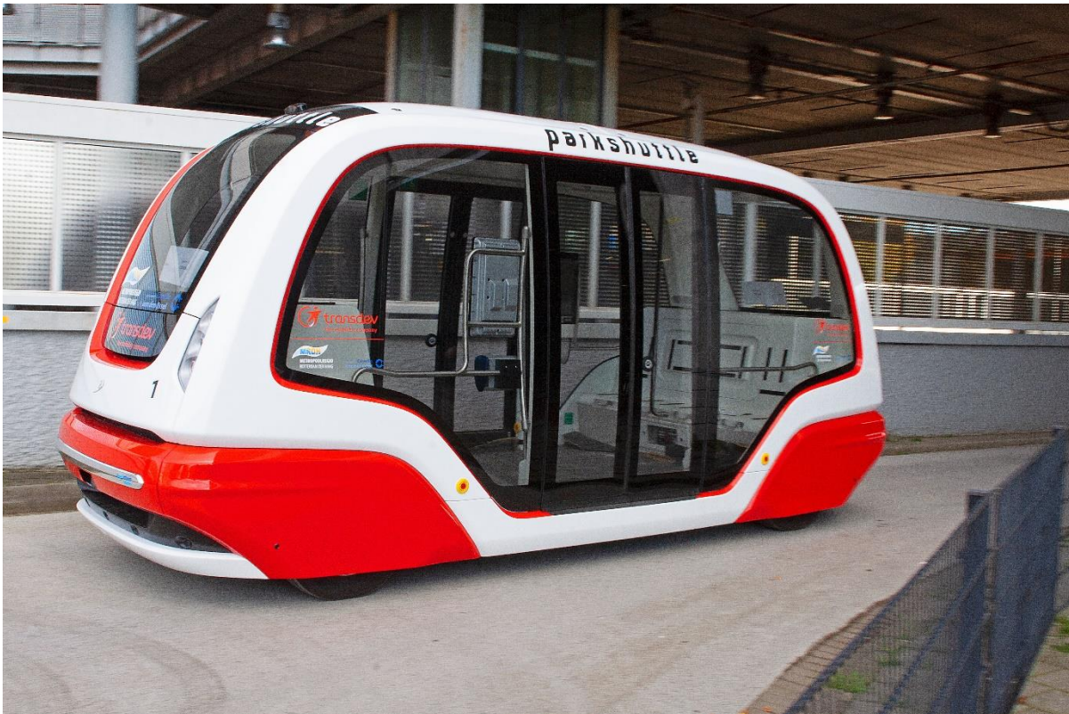
Figure 3. Exterior of a typical shuttle (2getthere) showing that the vehicle has very small wheels, two large outward folding glass doors on the side and is mostly designed for standing passengers as there is a relatively large open floor space.
