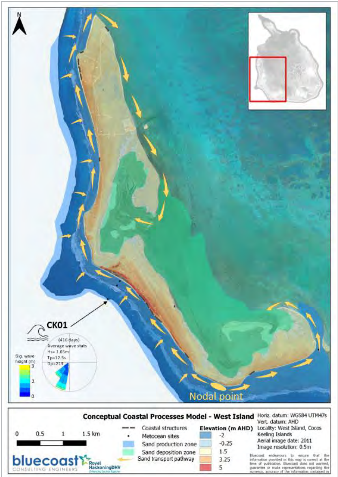
Figure 37: Conceptual coastal processes model, West Island (RHDHV, 2021a)
