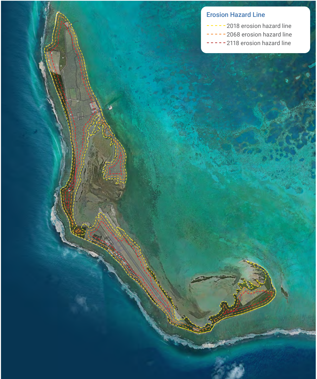
Figure 44: West Island erosion allowance
