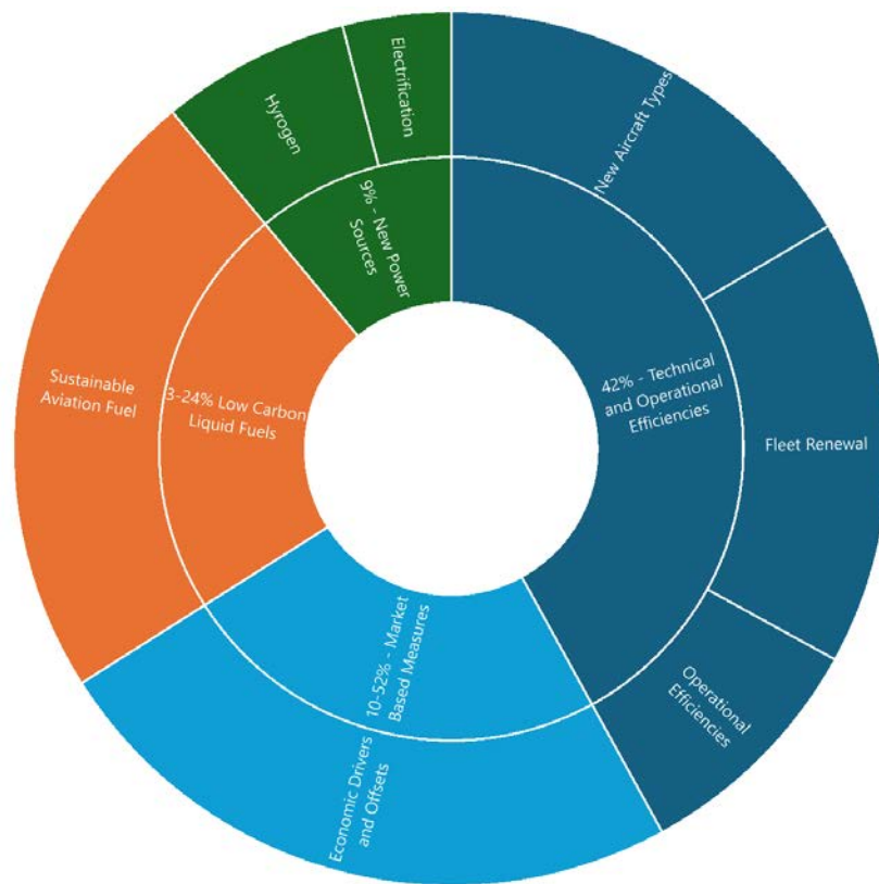
Figure 2: Potential CO 2 savings for the Australian aircraft fleet from different sources out to 2050 based on modelling of 2023 ADS-B flight data of the (combined domestic and international) VH-fleet
