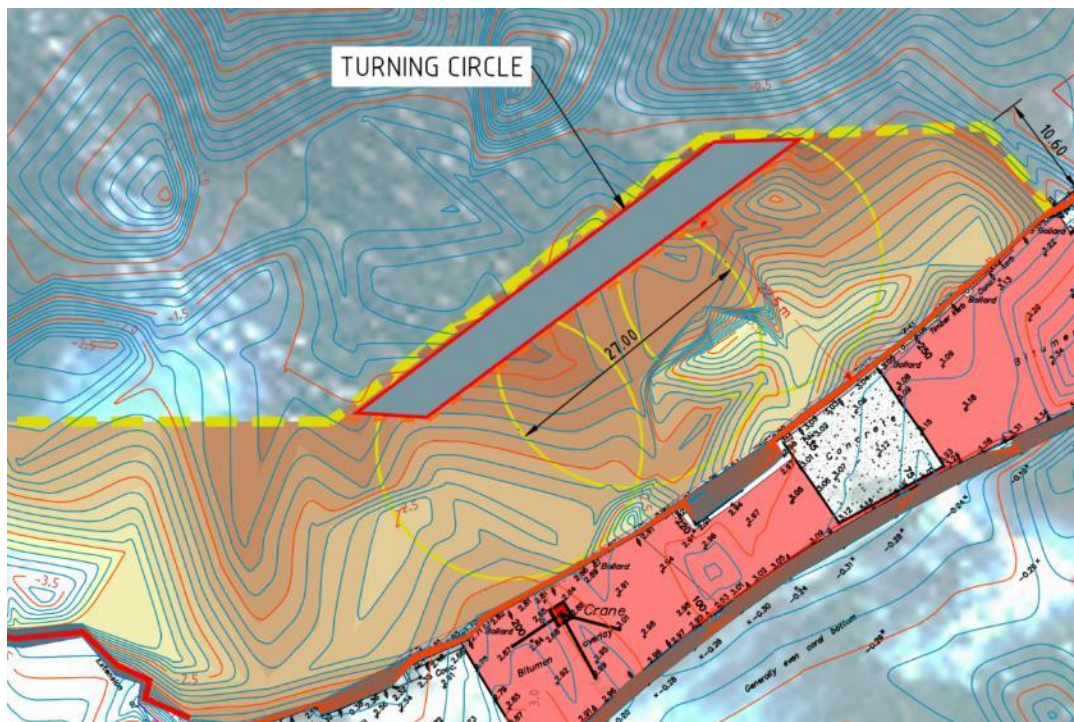
Figure 1-30 Option 3a reduced channel width (grey shading with red outline) compared to Option 3 (yellow dashed line).
