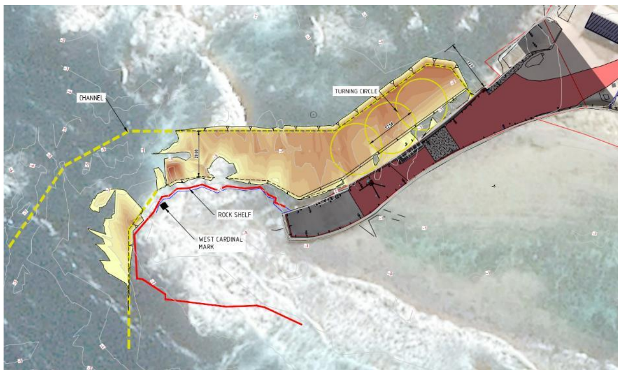
Figure 1-31 Preferred channel design alignment and volume cut.
