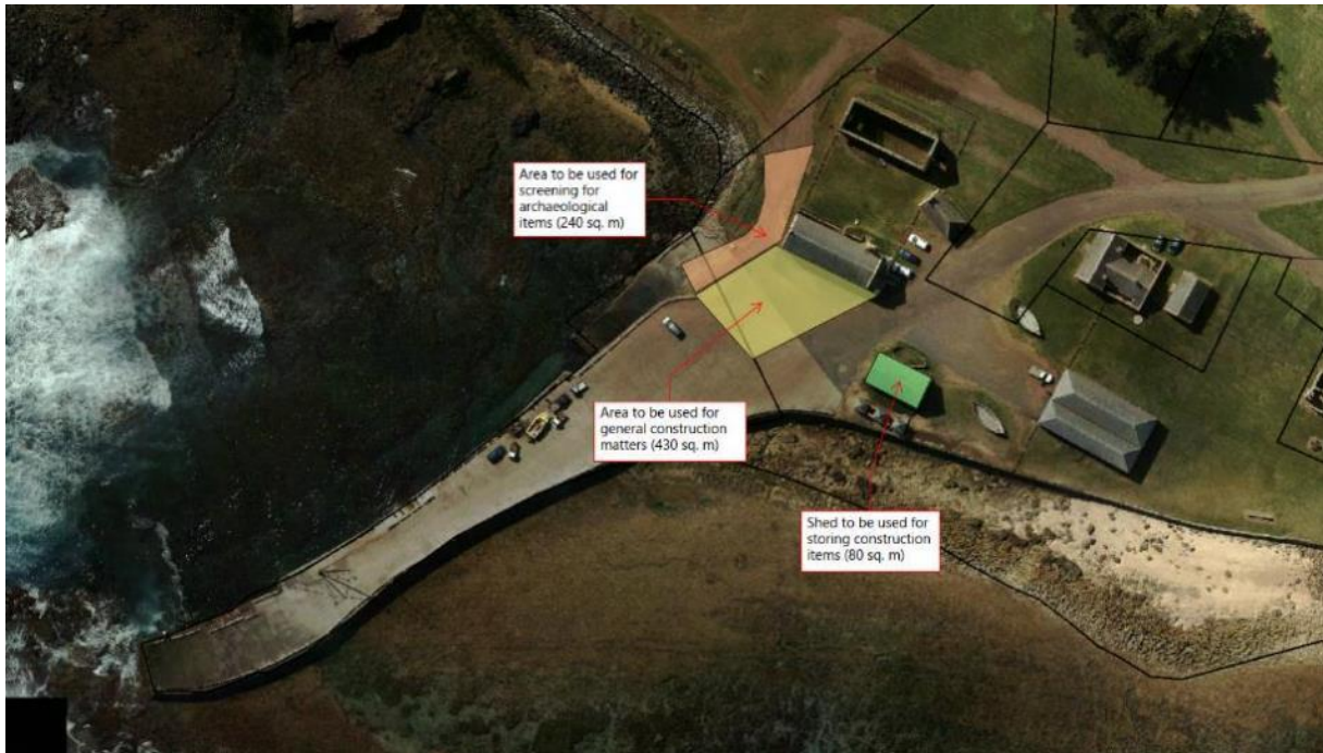
Figure 1-33 Contractor's site establishment.
