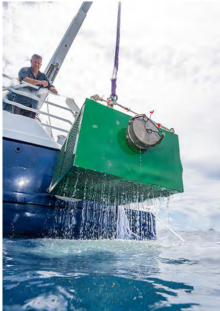
Figure 75 : Sediment box being lifted from seabed. (courtesy PDS)
