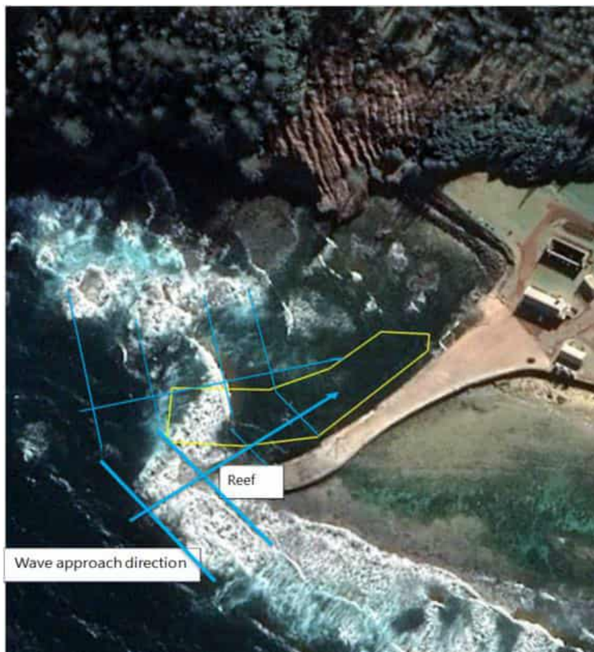
Figure 1-2 - Schematic of wave transformation paths that would be investigated following establishment of the nearshore wave climate.
