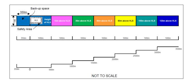
**Note:** Any development that exceeds the heights shown in Figure 1, which is consistent with the highest level of HLS classification (Performance Class 1), must be referred to the asset owner and CASA.
