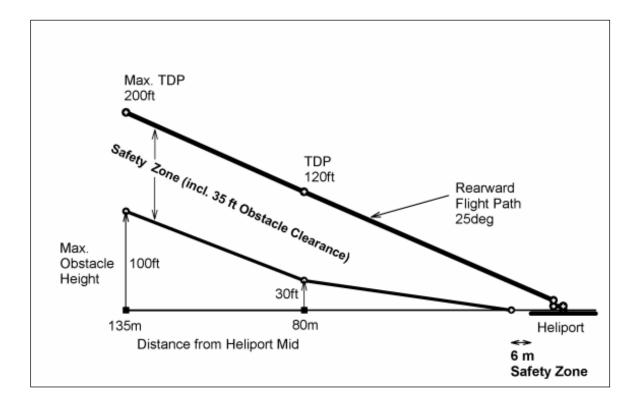
(Source: Eurocopter (now Airbus Helicopters) 'Figure C23 Rearward Flight Path (VTOL)', *Flight Manual EC* 135 P2+ Rev.10)
