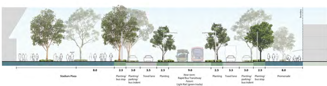
Figure 18. Example Transit Boulevard Section
