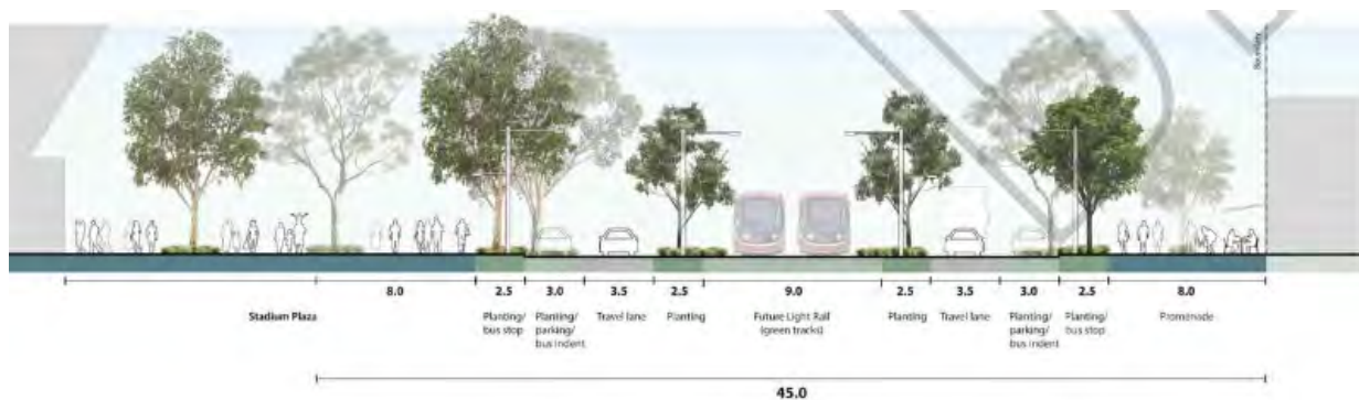
Figure 6-3 Example Transit Boulevard Section
