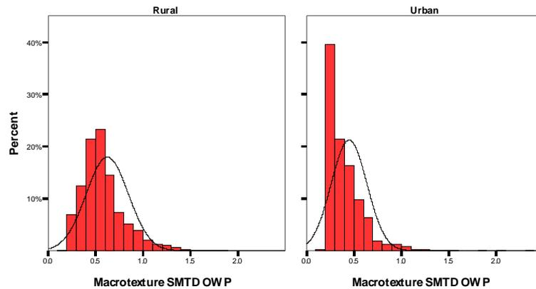
Figure 5: Macrotexture for rural and urban sections of the Great Eastern Highway, Direction 2.
