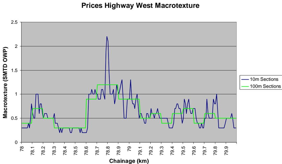
Figure 23: Macrotexture averaged over 10 m and 100 m sections, Princes Highway West.
