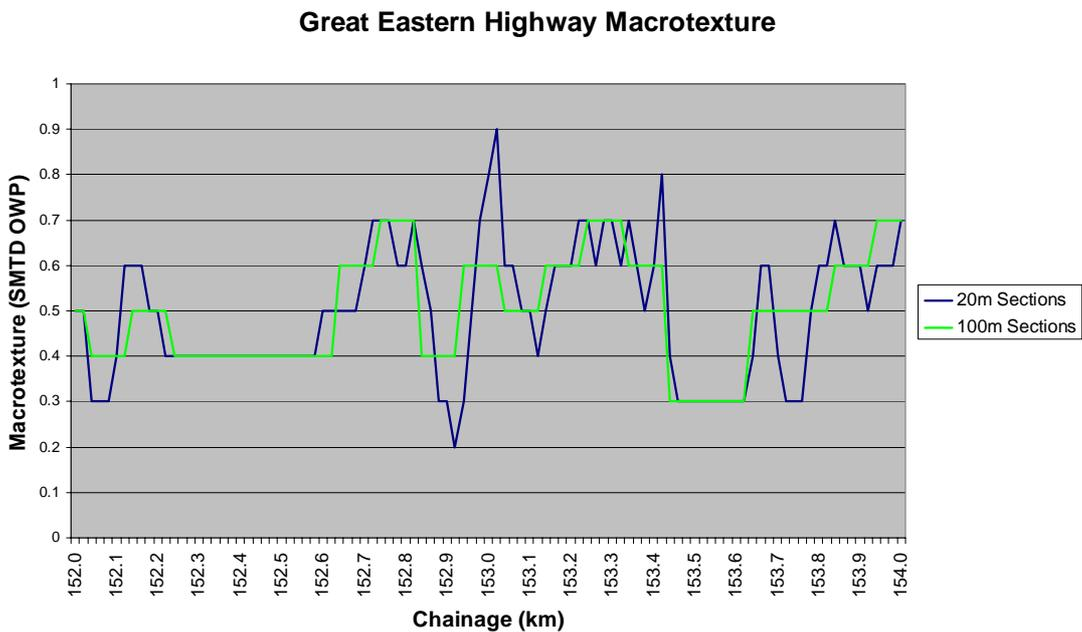
Figure 22: Macrotexture averaged over 20 m and 100 m sections, Great Eastern Highway.
