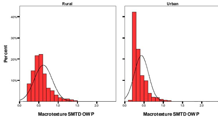
Figure 4: Macrotexture for rural and urban sections of the Great Eastern Highway, Direction 1.
