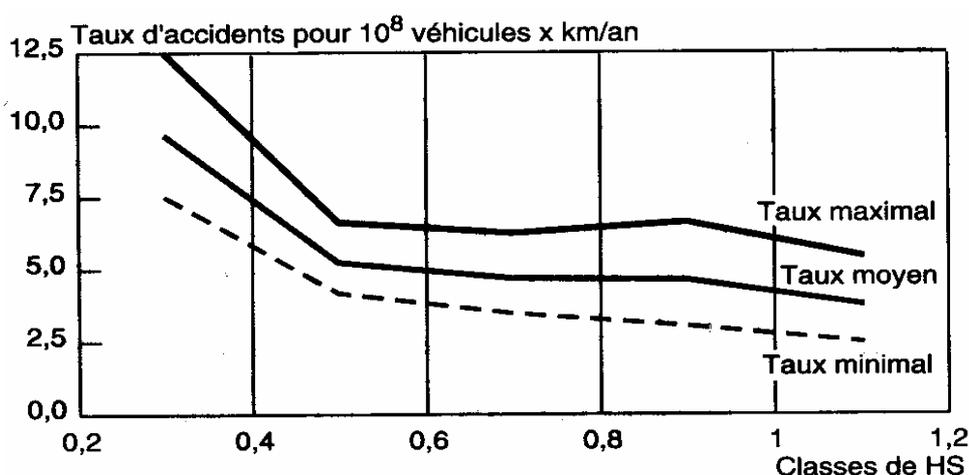
Figure 1: Relation between macrotexture and wet road crash rate (from Gothie 1993). The x-axis represents macrotexture, and the y-axis the wet road crash rate per 10<sup>8</sup> vehicle/km/year.
