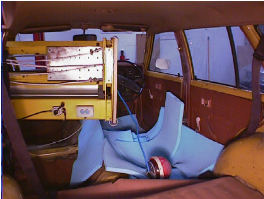
Figure 30. Test setup for B-pillar test. The photo was taken immediately after a test (Note that the RARU headform was used in the tests reported on in this report, not the EEVC WG10 headform as shown).
