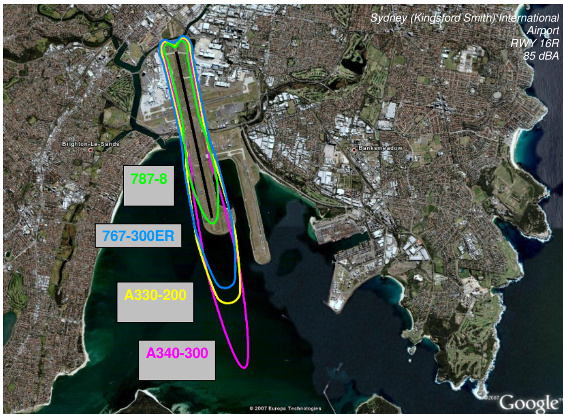
85 dB footprint of the 787 as compared to other aircraft
