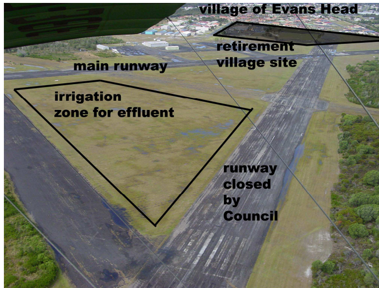
Figure 5: Area for irrigation of effluent is in the centre of the intersection of all four runways and is used by various aircraft. Proposed retirement village site shown in background. Irrigation of the area would have led to an increase in bird hazard and also introduction of 14 x 200mm high above-ground covers that would have been a hazard to aviation in the event of overrun or runoff or to existing users of the airfield.
